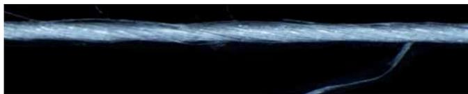
Figure 8. Yarn of intermediate entry compact spinning with suction groove spinning
