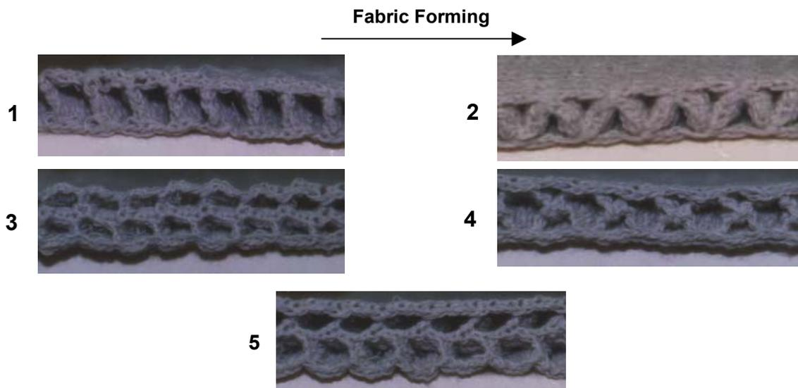
**Figure 6.** Multi-layered sandwich fabrics produced in a flat-bed knitting machine
