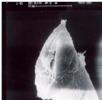
**Figure 8.** SEM Photo of broken filament
