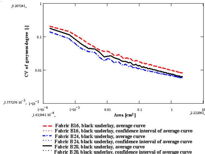
Figure 1. Average external area-variation curves - fabrics B16, B20, and B24, black underlay.
