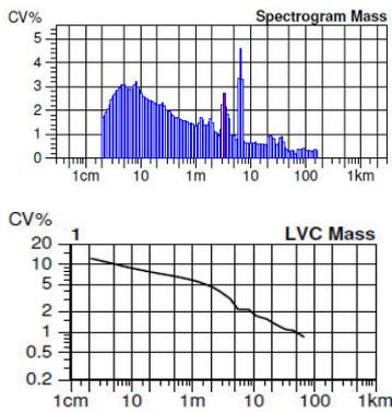
Figure 3. Spectrogram and variance length curve - yarn No. 1.
