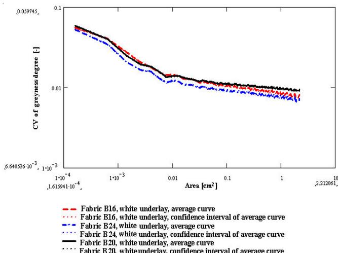
Figure 2. Average external area-variation curves - fabrics B16, B20, and B24, white underlay.
