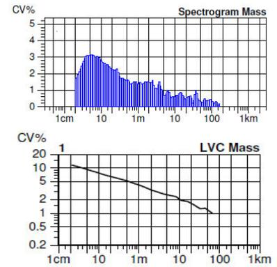
Figure 5. Spectrogram and variance length curve - yarn No. 4.
