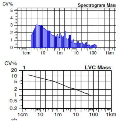
Figure 4. Spectrogram and variance length curve - yarn No. 5.
