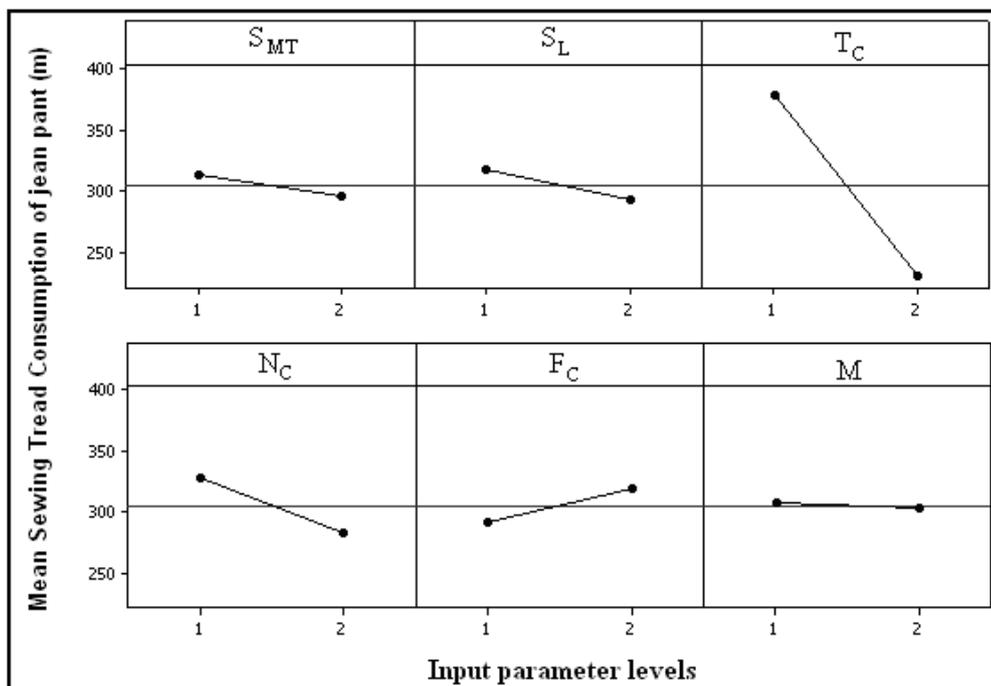
Figure 3. Mean variation of sewing thread consumption as function of studied input parameters given by Minitab software.
