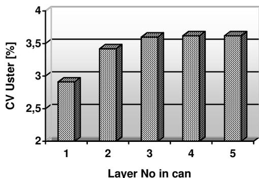
Figure 5. CV Uster (%) of "autolevelled" card sliver in the successive layers in the can (numbered from the top of the can).
