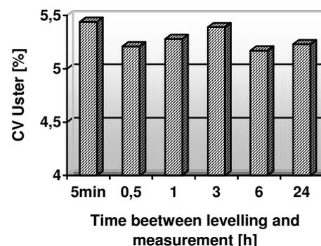
Figure 8. CV Uster (%) of "unautolevelled" card sliver determined at various times after passing through a leveller.
