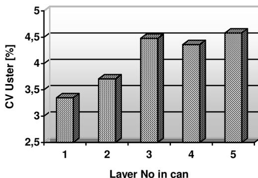
Figure 6. CV Uster (%) of "autolevelled" card sliver in the successive layers in the can (numbered from bottom of the can).
