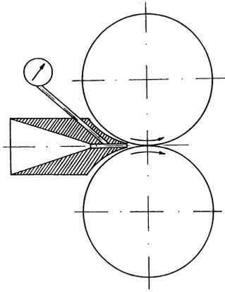
Figure 3. A diagram of the active pneumatic measurement system.
