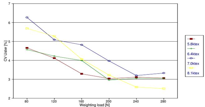
Figure 4. Autolevelled card sliver irregularity as a function of weighting load applied to the measuring roll.
