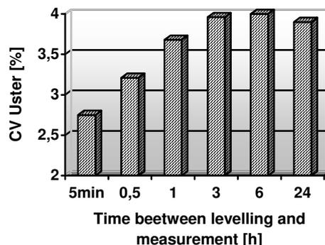
Figure 7. CV Uster (%) of "autolevelled" card sliver determined at various times after levelling.
