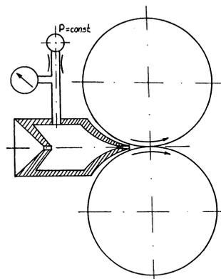
Figure 2. A diagram of the passive pneumatic measurement system.
