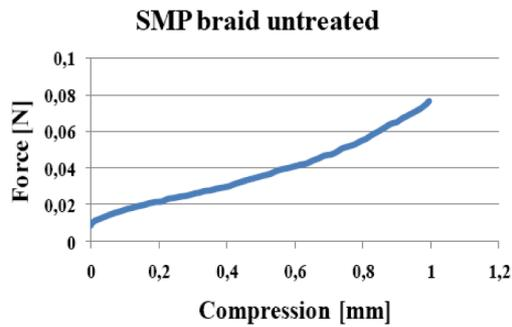
Diagram 3. Pinching test results (compression 1 mm) of an untreated SMP braid.
