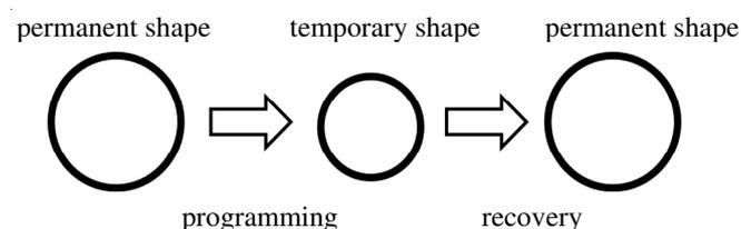
**Figure 1.** Schematic view of the thermally induced shape memory effect.
