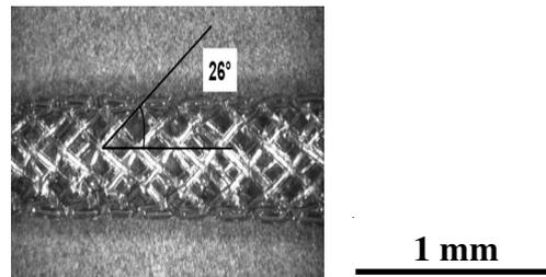
**Figure 3.** 16 filament SMP braid on a mandrel.
