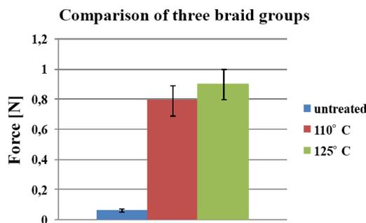
Diagram 5. Comparison of the three different braid groups. Untreated and treated at 110°C and 125°C for 10 minutes with a 1 mm radial compression.
