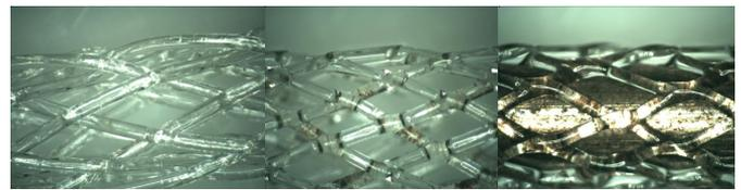
**Figure 7.** Microscopic pictures of SMP braids (from left to right) heat-treated at 70°C, 125°C and 150°C for 10 minutes.
