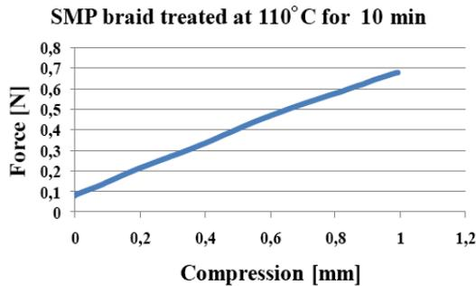
Diagram 4. Pinching test results (compression 1 mm) of a heat-treated SMP braid at 110°C for 10 min.
