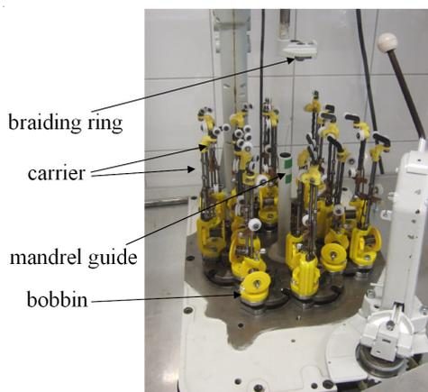
**Figure 2.** 16 carrier circular braiding machine.
