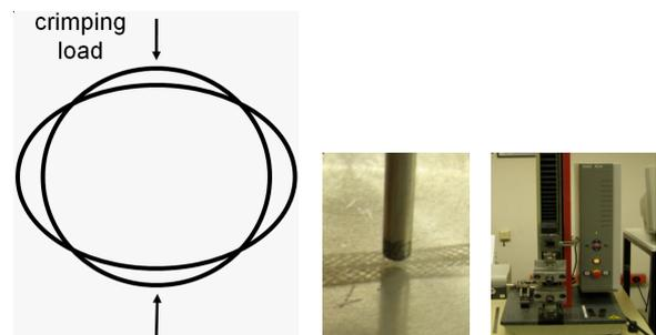
**Figure 5.** Crimping load (left), crimping test of the SMP braid (middle), tensile testing machine Z 2.5 Zwick GmbH (right).
