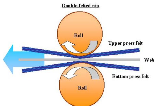
**Figure 1.** This nip builds up about two rolls and two press felts.
