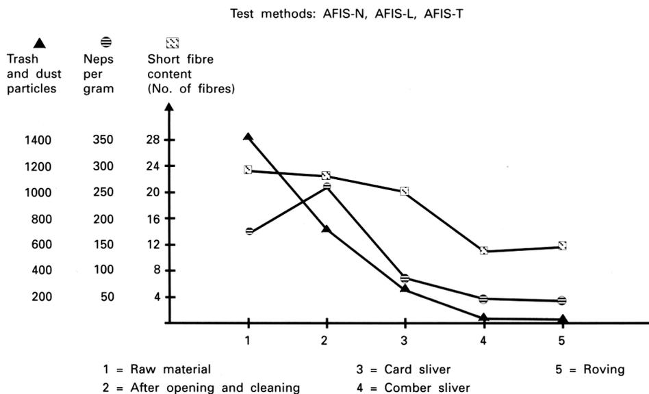
Figure 5. Process analysis in a spinning mill
