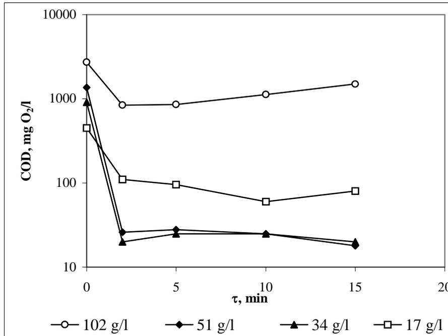
**Figure 3.** Dependence of COD of water polluted with different oil concentrations by using of THL sorbent on the duration of the sorbent action
