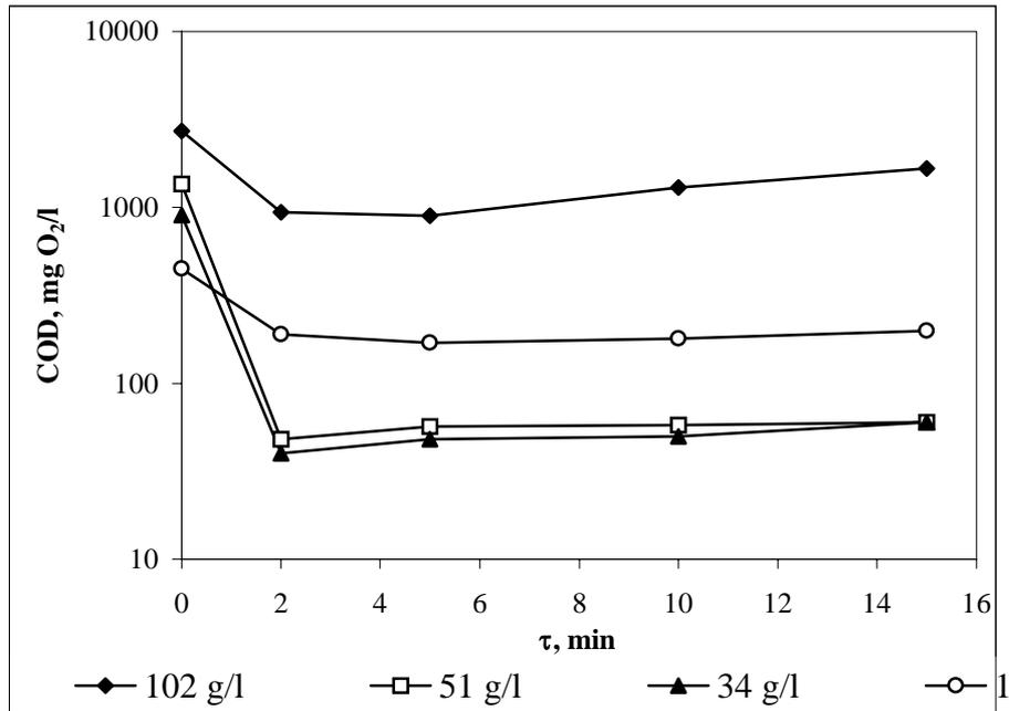
**Figure 5.** Dependence of COD of water polluted with different oil concentrations by using of wood barks sorbent on the duration of the sorbent action
