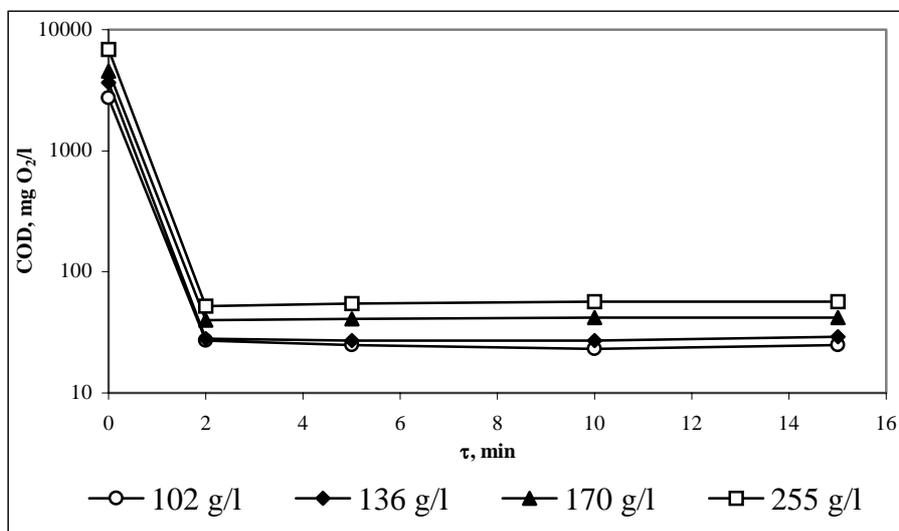
**Figure 1.** Dependence of COD of water poluted with different oil concentrations by using of wool shoddy sorbent on the duration of the sorbent action
