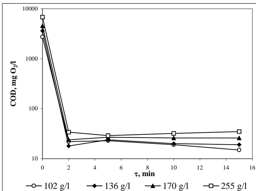
**Figure 2.** Dependence of COD of water poluted with different oil concentrations by using of art. Druzeta sorbent on the duration of the sorbent action
