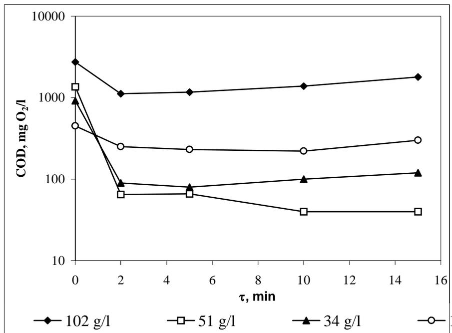
**Figure 4.** Dependence of COD of water polluted with different oil concentrations by using of wood saw-dusts sorbent on the duration of the sorbent action
