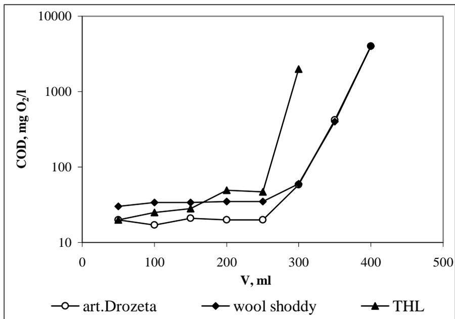
**Figure 6.** Dependence of COD of water polluted with oil by cleaning with wool shoddy, art. Drozeta and THL at dynamic condition on the volume of liquid
