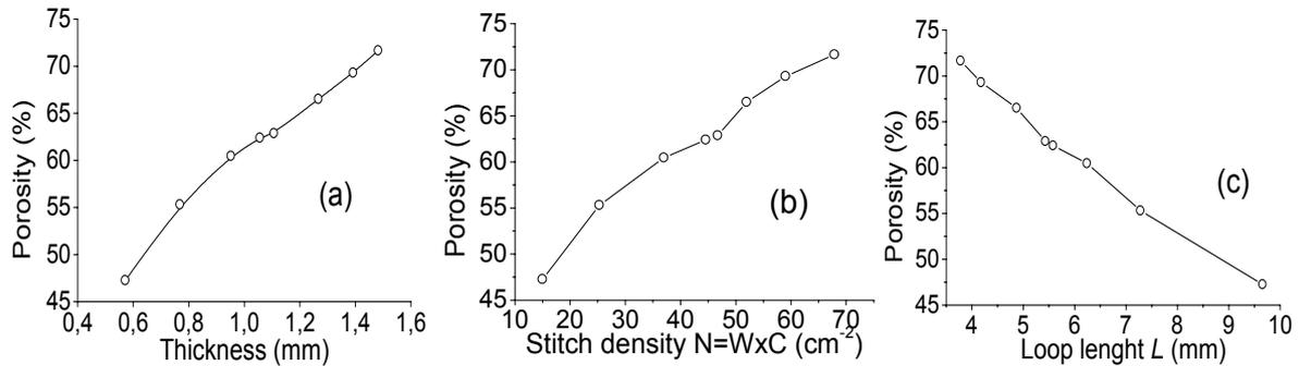
**Figure 9.** Knitting parameters' influence on porosity
