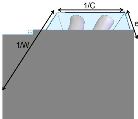
**Figure 4.** Three-dimensional elementary jersey loop shape
