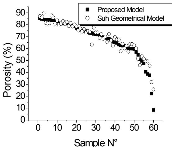
**Figure 5.** Porosity values using geometrical modelling Comparing the methods of image processing, geometrical modelling (Equation 5) and that using air permeability, we obtain the result mentioned in Figure 6. Experiments were carried out on 60 samples divided according to various gauges (5, 7, 12, and 24) and different knitting parameters.
