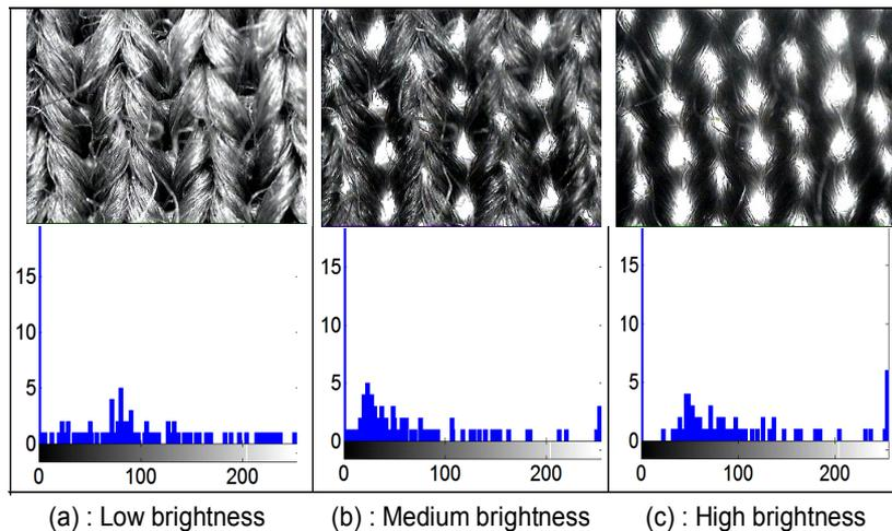
Figure 7. Light intensity's influence on pore shape
