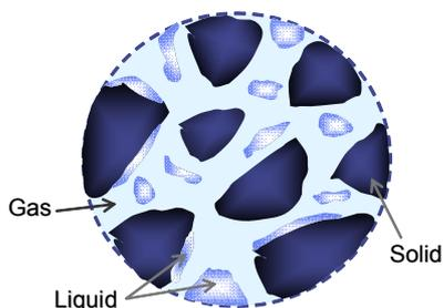
**Figure 1.** Geometry of a porous medium
