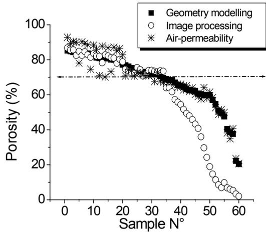
Figure 6. Porosity values according to various methods
