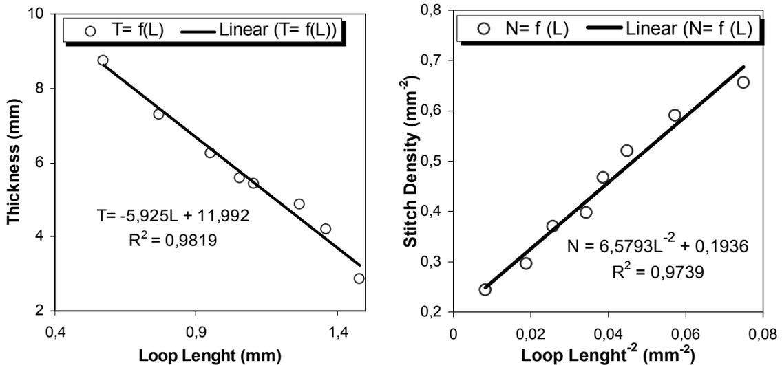
**Figure 10.** Variation of thickness (T) and stitch density (N) according to the loop length (L)
