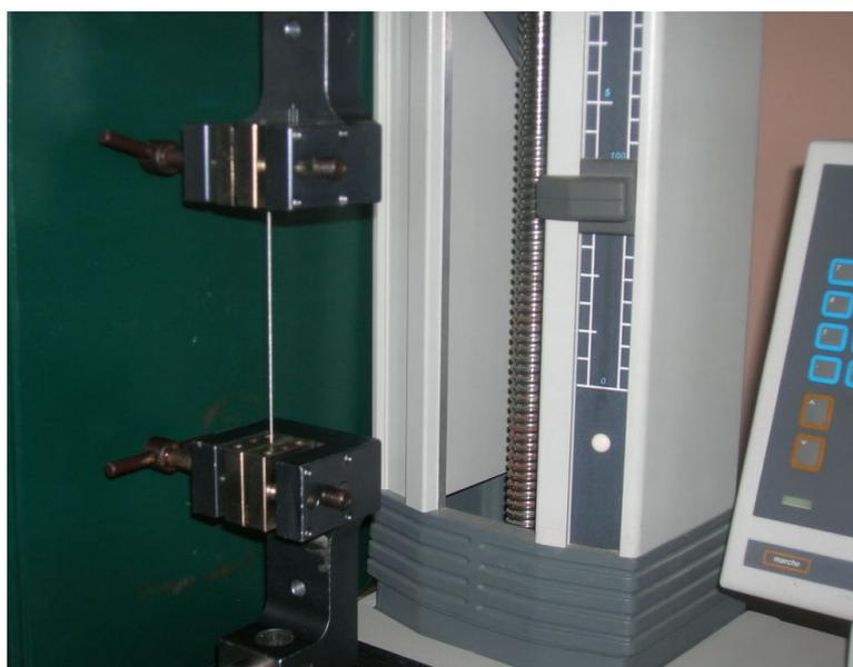
**Figure 2.** Dynamometer for breaking strength measurements
