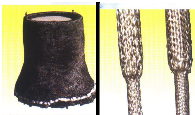
Figure 2. Some samples of 3-D braided perform
