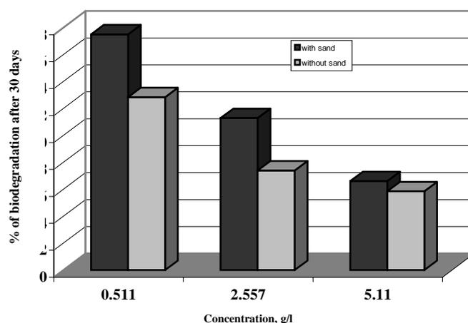
**Figure 7.** Influence of the presence of sand on the biodegradation
