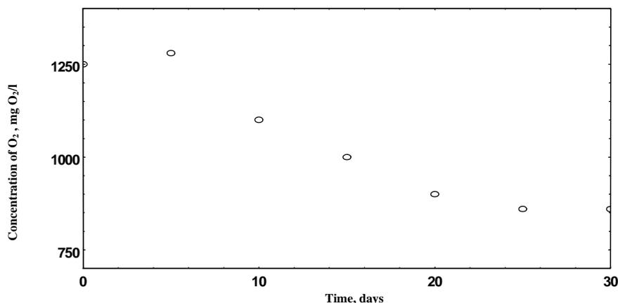
Figure 4. Evolution of COD versus time (concentration 0.511 g/l)
