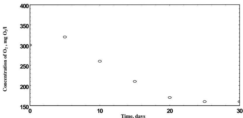
Figure 3. Evolution of COD versus time (concentration 0.102 g/l)
