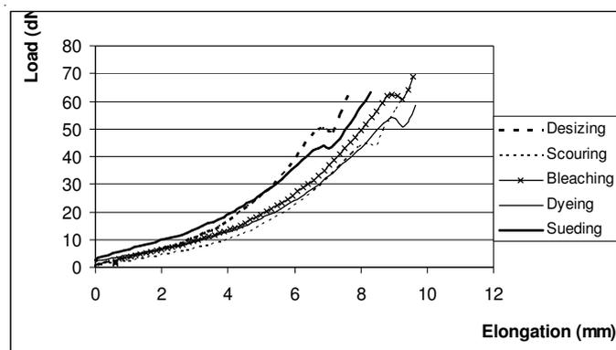
Figure 11. Load-elongation for seam in warp direction.
