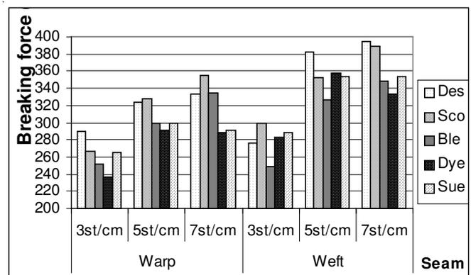
Figure 8. Breaking force for different density for all treatment.
