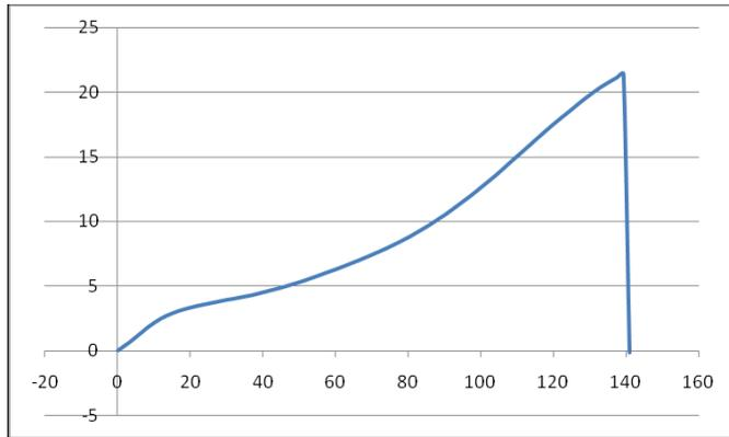
**Figure 4.** Strength[N]/elongation[mm] curve of sewing yarn before sewing.
