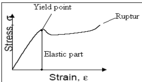
Figure 10. Strain-stress curve for elastic material.
