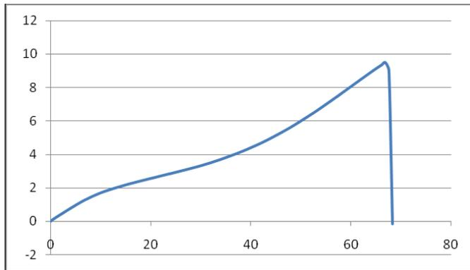
**Figure 5.** Strength[N]/elongation[mm] curve of sewing yarn loop.
