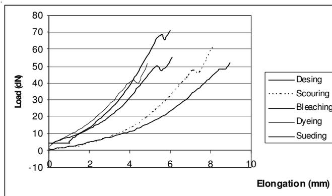
Figure 12. Load-elongation for seam in weft direction.
