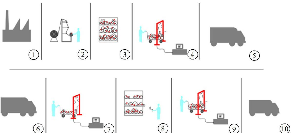
Picture 5. Example of RFID application in a textile factory where: 1 – production, 2 – standardization section, preparation of fabric for ready use, labelling the fabric with RFID tag, 3 – stock-room, 4 – RFID pike monitors fabric release, 5 – transportation of fabrics, 6 – delivery of fabrics to a wholesaler, 7 – acceptance of fabrics at RFID pike, 8 – wholesale stock-room, 9 – release of fabrics at RFID pike, 10 – transportation.
