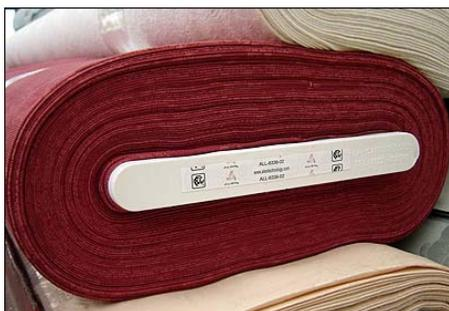
Picture 6. Roll of fabric with RFID tag attached [19].
