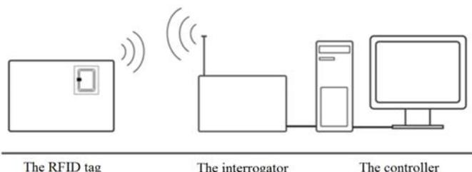
Picture 1. Scheme of RFID system.
