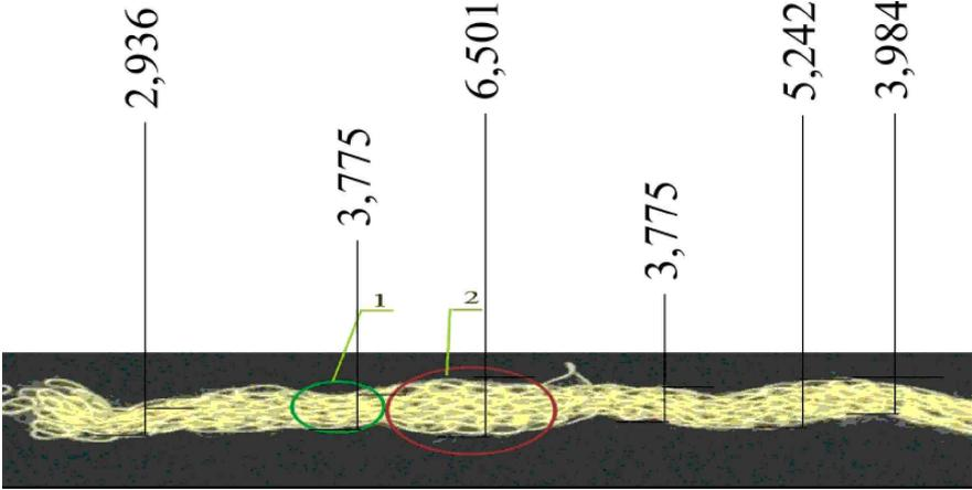
**Figure 3.** The yarn-band after knitting and unknitting with visible changes of its structure
