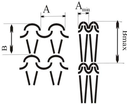
**Figure 2.** Stitch image of plain knit right-side knitting: a) in balanced state, b) at maximal stretching on length (per stitch rows)
