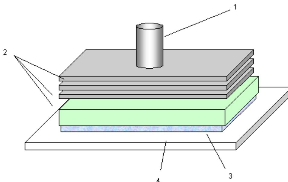
**Figure 7.** Schematic of test apparatus for acquisition, rewet and wicking distance tests.
