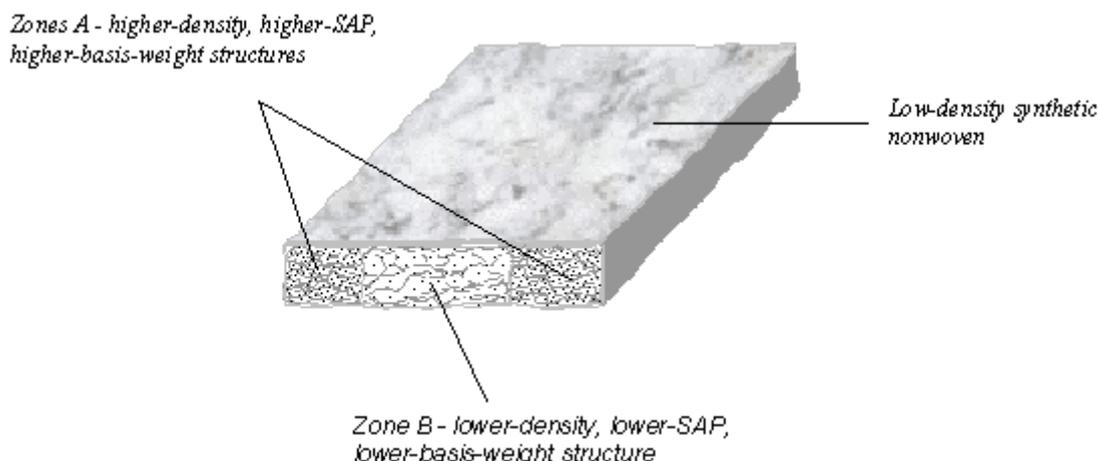
**Figure 10.** Schematic view of unitary ASP structure with y-directional gradient in density, basis weight and SAP content [8]
