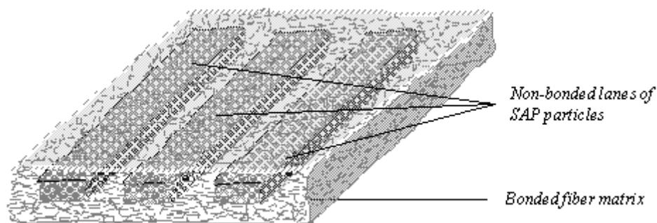
**Figure 11.** Schematic view of unitary structure with less bonded lanes of particles enclosed within well bonded fiber network [5]
