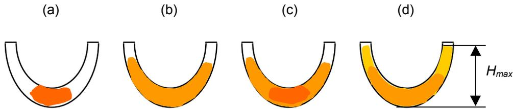
**Figure 1.** Progressive distribution of acquired liquid in absorbent system due to wicking against gravity (darkness of colored areas represent concentration of liquid):
