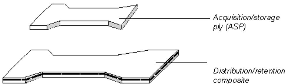
**Figure 6.** Exploded, perspective view of the components of an absorbent system comprising ASP structure as described in reference [5]
