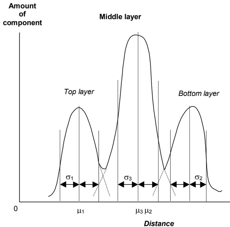
**Figure 9.** An example of contact intimacy in a three-layer structure [7]
