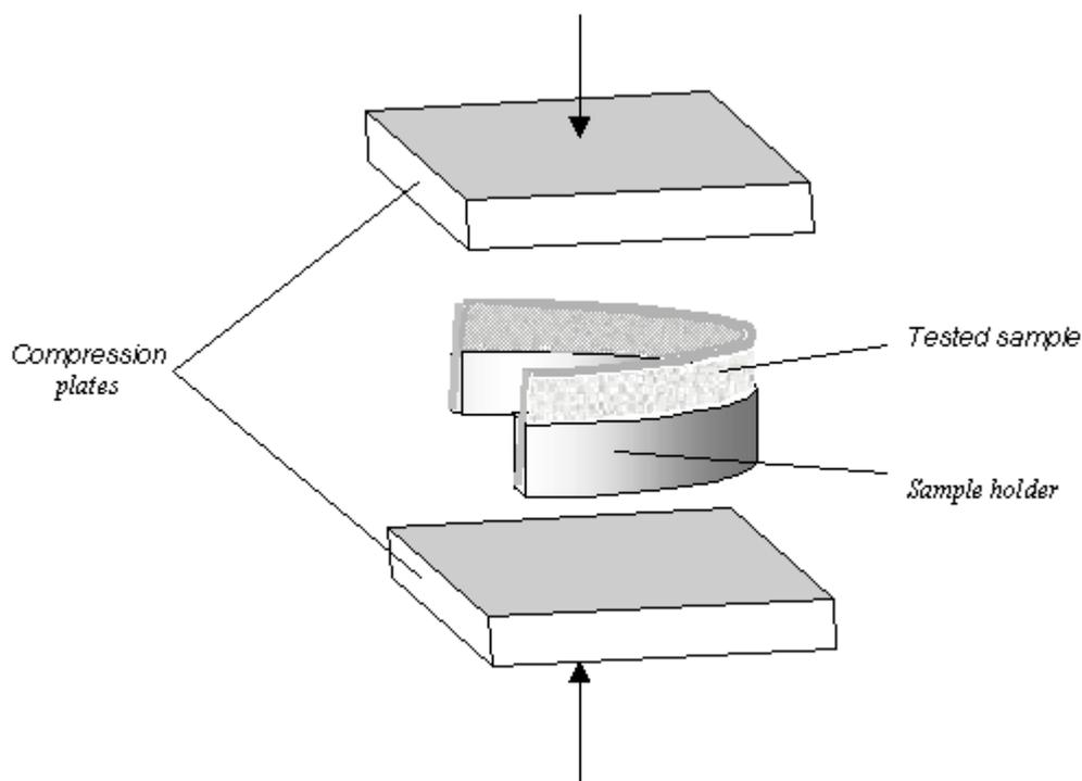
**Figure 12.** Measurement of CD softness according to reference [5]
