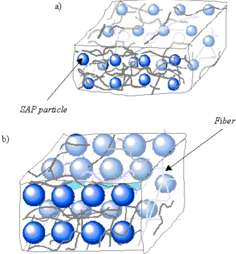
**Figure 3.** Ideal composite with uniformly arranged SAP particles: a) in dry state; b) with swelled SAP particles
