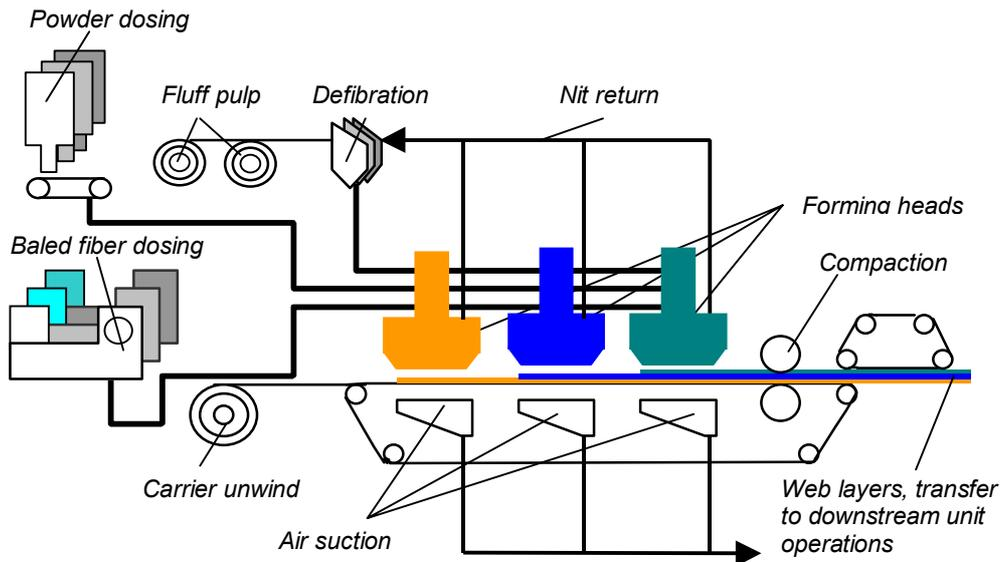
**Figure 8.** Schematic of the web-forming stage of the airlaid process
