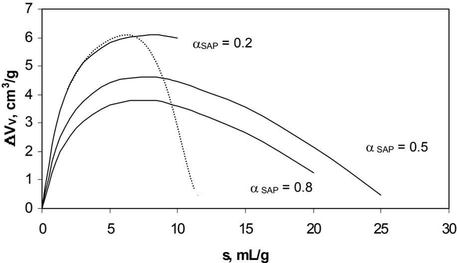
**Figure 4.** Changes in void volume in fiber/SAP composites in function of web saturation. Dotted curve based on data by Sawyer *et al.* [3]
