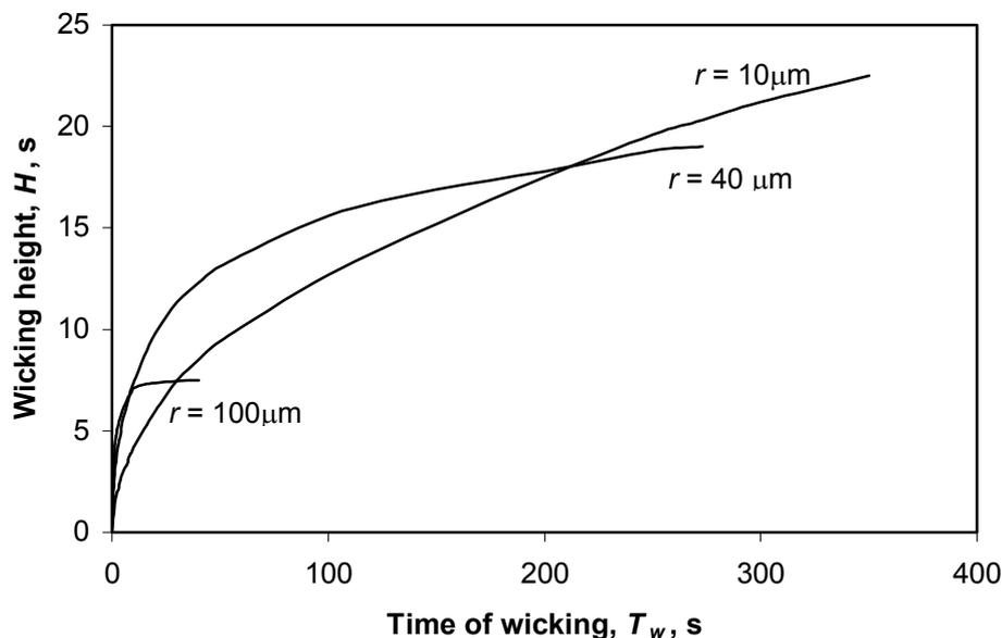
**Figure 2.** Vertical wicking of liquid in porous cellulose web, based on equation (2). Liquid parameters (as for 0.9% saline):  $\gamma = 75$  dynes/cm;  $\eta = 1$  centipoise;  $\Psi = 75$  m/s; advancing contact angle  $\Theta_A = 60^\circ$
