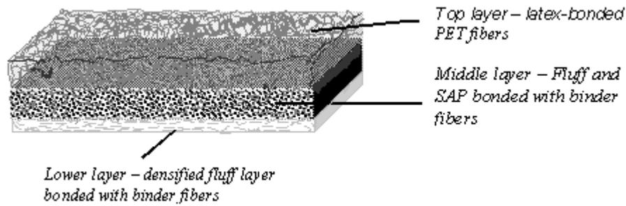
**Figure 5.** Schematic view of multilayer unitary ASP structure with z-directional density gradient for controlled fluid flow [5]
