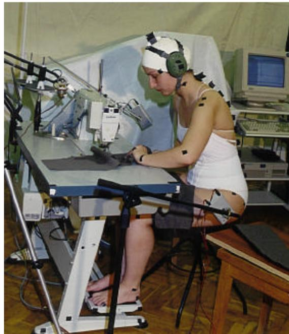
**Figure 4:** Body posture with marks, in the course of sewing the second segment of the seam (Fig. 3 - segment 4)
