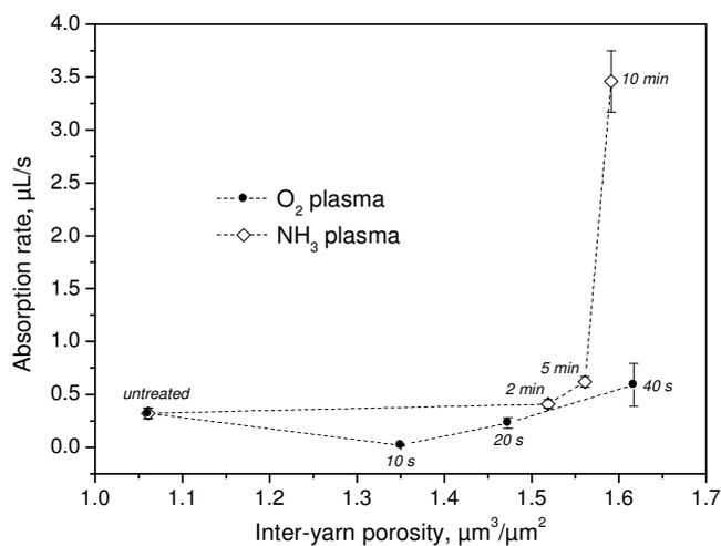
**Figure 14.** Effect of inter-yarn porosity on the absorption rate of 10µL water drops.
