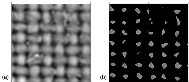
**Figure 7.** Inter-yarn porosity was calculated using the parameter 'lubricant filled profile valley area' extended to 3D-topography. (a) topographical contrast map, (b) the same map after isolating the inter-yarn pores.
