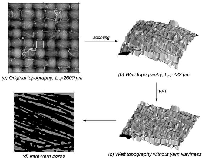
**Figure 9.** Quantification of intra-yarn porosity: (a) yarns must be zoomed out from the original topographic map, (b) yarn topography includes the curvature due to yarn profile, (c) this curvature is removed using Fast Fourier Transformations, (d) the intra-yarn porosity can be quantified using the algorithm 'lubricant filled profile valley area'.
