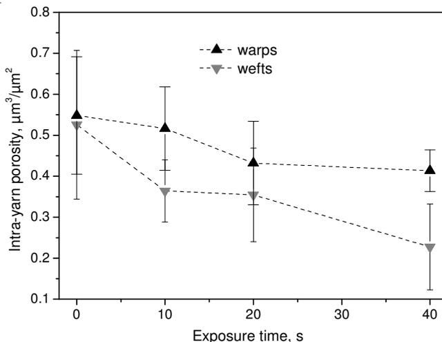
**Figure 10.** Effect of treatment with O<sub>2</sub>-plasma on intra-yarn porosity.
