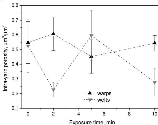
**Figure 11.** Effect of treatment with NH<sub>3</sub>-plasma on intra-yarn porosity.
