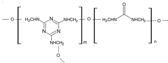
Figure 1. General structure of the dye fixer.
