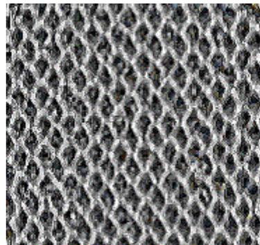
**Figure 4b.** The result of glass fiber preform surface image using median filter algorithm of mathematical morphology
