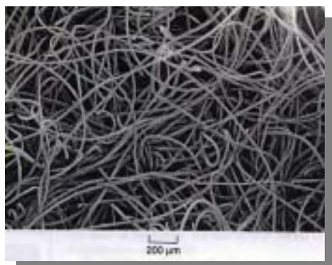
Figure 2. SEM of nonwoven PGA scaffold
