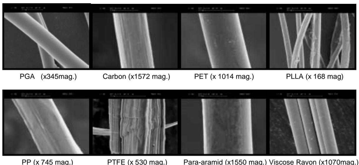
**Figure 3.** SEM images illustrating the surface topography of generic fibres used in the biocompatibility experiment
