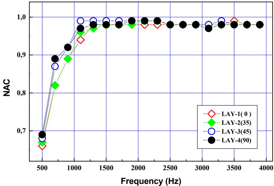
Figure 3. Effect of mid-web angle on sound absorption properties
