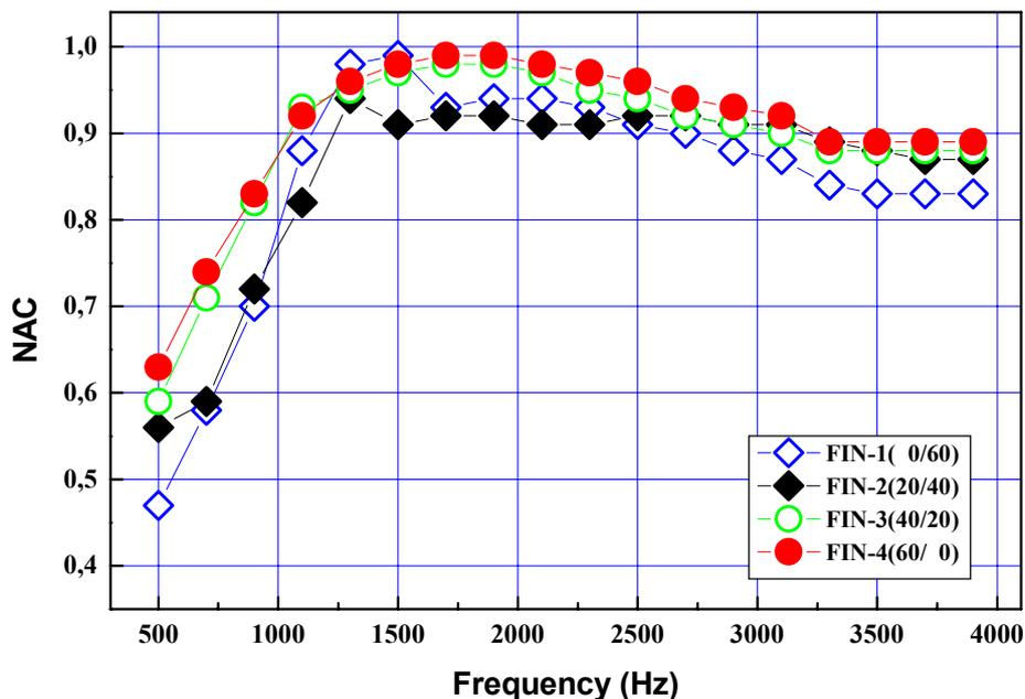
**Figure 1.** Effect of fine fibre contents on sound absorption properties
