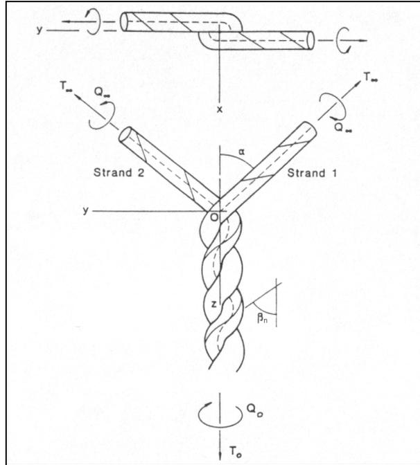
**Figure 3.** Schema of a twisted multi-folded thread accepted for consideration, and presented in the Cartesian co-ordinate system [3]
