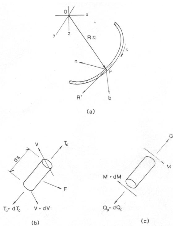
Figure 5. Schematic drawings presenting: twisted together, and presented a) Position of the radius vector  $R(s)$ , the normal in the Cartesian co-ordinate system [4] main vector  $n$ , and the bi-normal vector  $b$ ; b) forces acting on an element of the component fibre stream; c) momenta acting on an element of the component fibre stream [3, 4]
