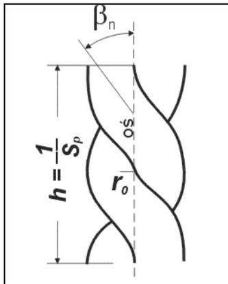
**Figure 1.** Schema of a twisted multi-folded thread (doubled yarn) accepted for consideration [12, 13]
