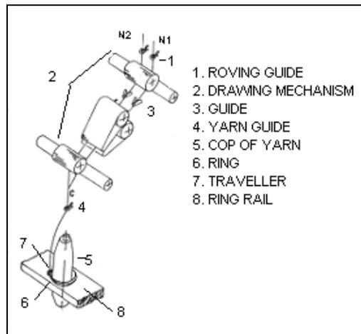
**Figure 2.** Schema of the twisting-and-spinning mechanism of a ring spinning frame [4]
