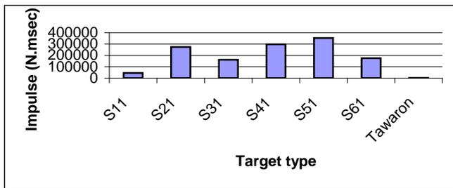
**Figure 10.** Impulse via different composite panel types (at 1.5 J).
