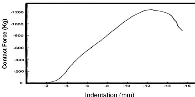
Figure 17. Force-indentation response in contact loading of panel S2.
