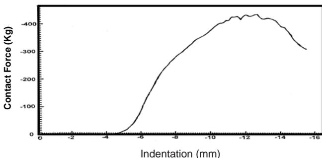
Figure 16. Force-indentation response in contact loading of panel S1.
