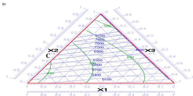
Figure 15. Overlap of peak dynamic force (—) and impulse (---) contours of straw composite panels at 3 J.
