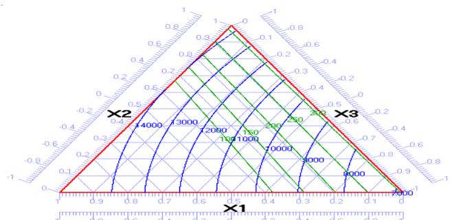
**Figure 14.** Overlap of peak dynamic force (—) and impulse (---) contours of straw composite panels at 2.25 J.
