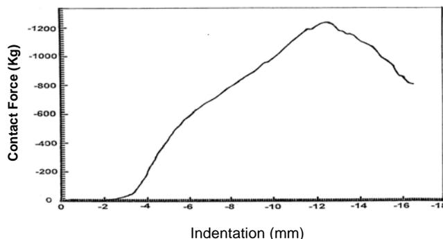
Figure 18. Force-indentation response in contact loading of panel S3.
