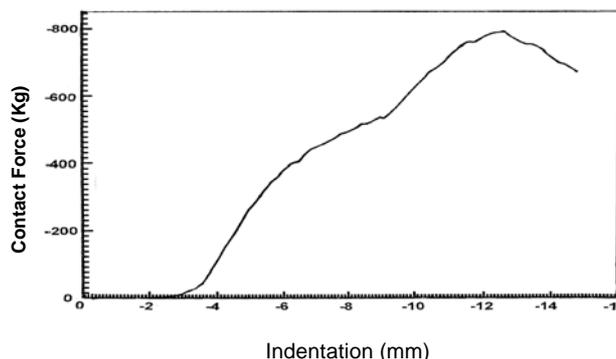
Figure 20. Force-indentation response in contact loading of panel S5.
