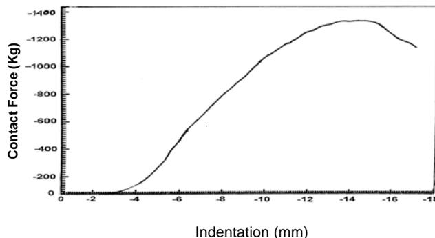
Figure 19. Force-indentation response in contact loading of panel S4.
