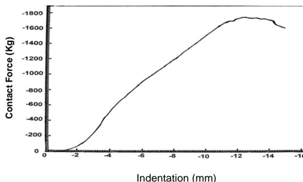
Figure 21. Force-indentation response in contact loading of panel S6.
