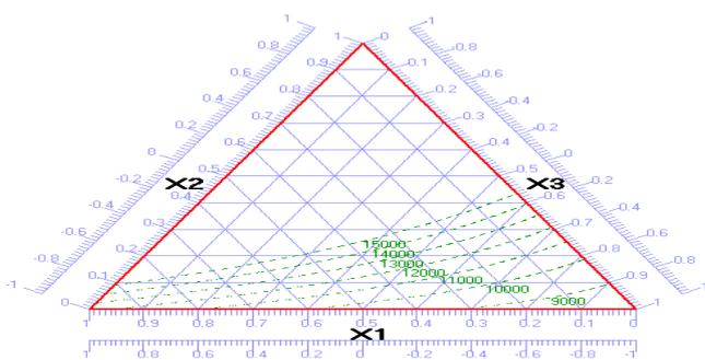
**Figure 23.** Absorbed energy contours of straw composite panels.
