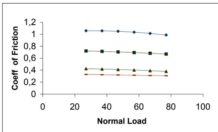
**Figure 2b.** Coefficient of friction of fabrics as a function of normal load at an area of 11.5 cm<sup>2</sup>
