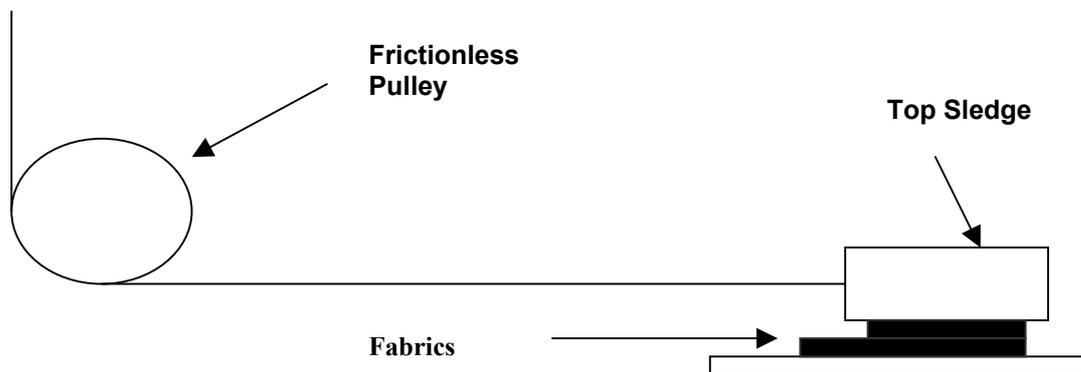
Figure 1. Frictional set-up used in Instron for testing friction
