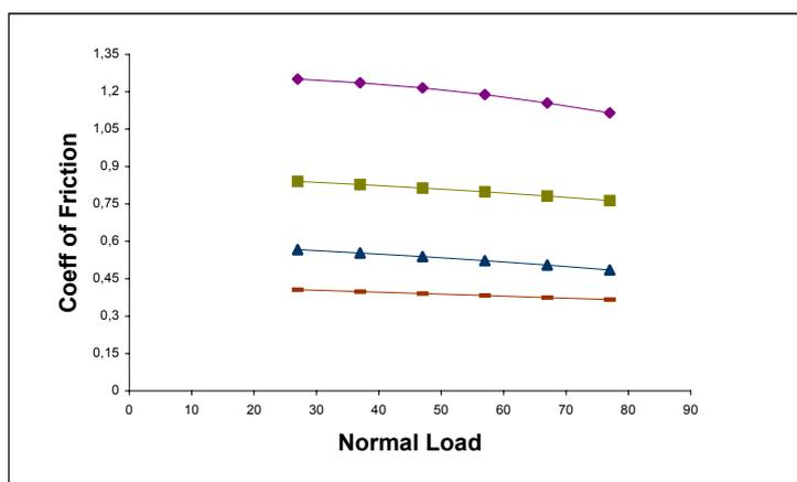
**Figure 2a.** Coefficient of friction of fabrics as a function of normal load at an area of 13.3 cm<sup>2</sup>
