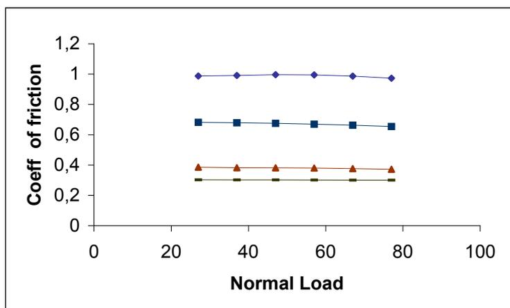
**Figure 2c.** Coefficient of friction of fabrics as a function of normal load at an area of 9.7 cm<sup>2</sup>
