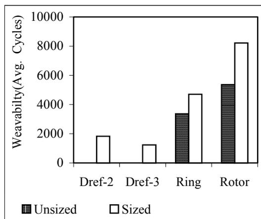
**Figure 4.** Effect of Starch/Acrylic Size on weavability of Dref-2 and Dref-3 yarns at High Add-on
