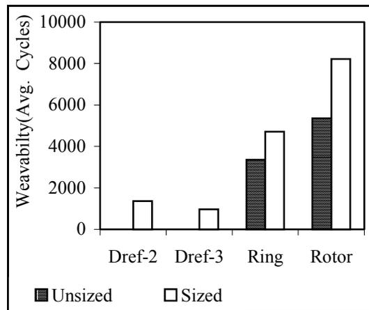
Figure 3. Effect of normal Starch Size on weavability of Dref-2 and Dref-3 yarns at High Add-on
