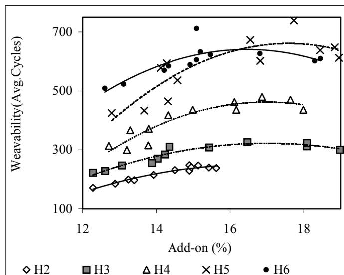
Figure 1. Effect of Add-on on Weavability of Dref yarns with Filament Core
