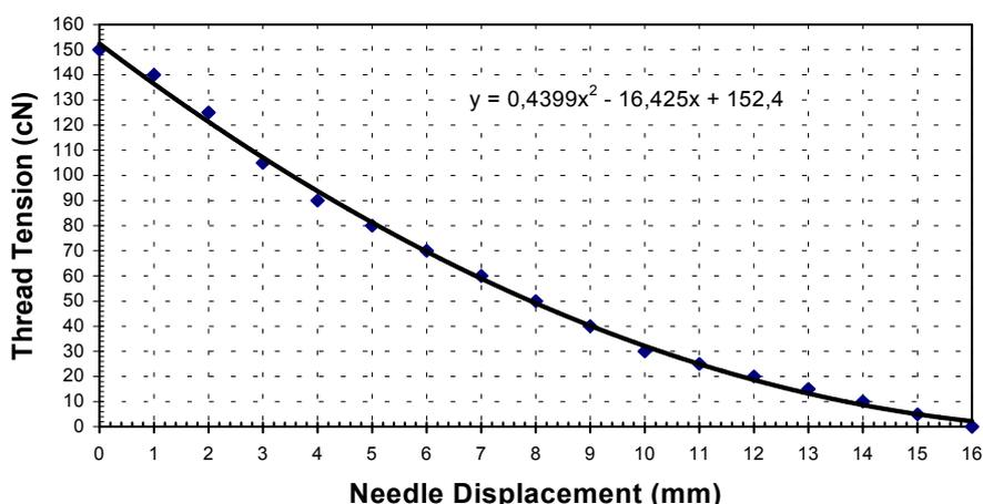
**Figure 3.** Force-displacement depending calibration curve
