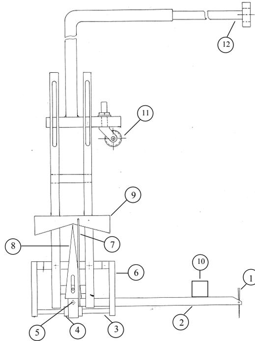
**Figure 1.** Needle-mechanical device
