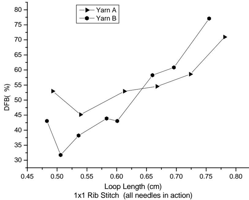
**Figure 4.** Variation of DFB in term of the loop length for 1 × 1 Rib II (all needles in action)
