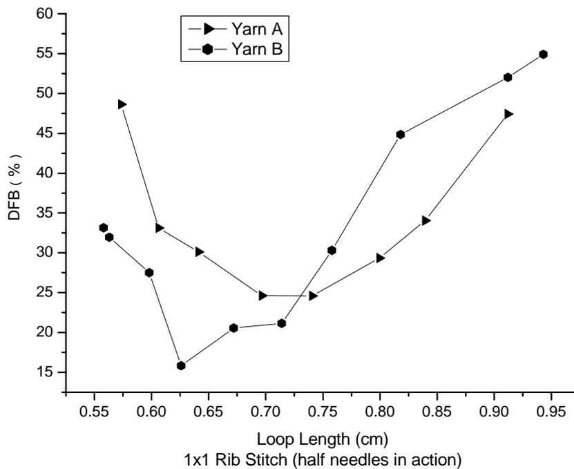
Figure 3. Variation of DFB in term of the loop length for 1 x 1 Rib I (half needles in action)
