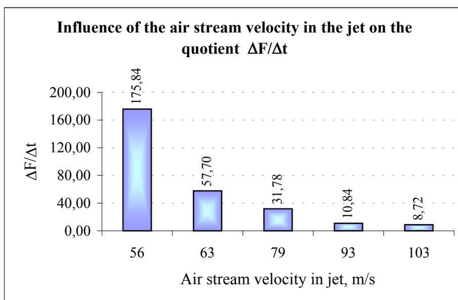
**Figure 9.** Dependence of  $\Delta F/\Delta t$  for roving with 135 twists/m on the air stream velocity
