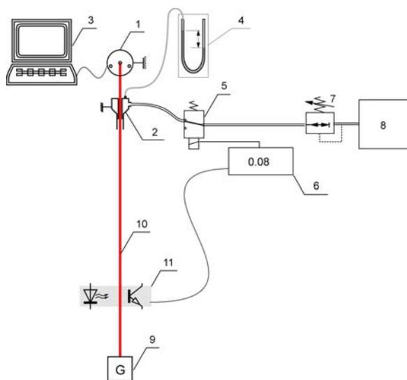
**Figure 5.** Measuring stand for dynamic stretching; 1 – tension gauge for the sample tested, 2 – jet, 3 – computer-aided measuring and control system, 4 – manometer, 5 – electrically controlled valve, 6 – time-lag switch, 7 – pressure reducer (controller), 8 – compressor, 9 – breaking load acting over free falling ( $h = 2\text{ m}$ ,  $G = 200\text{ g}$ ), 10 – sample tested, 11 – photo-optical sensor which releases the air stream in the jet (with programmed time-span).
