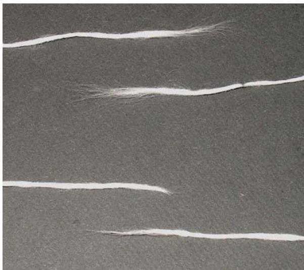
**Figure 11.** Photographs of the roving ends after destruction; from above: continuity loss by defibration of a roving with 95 twists/m, and continuity loss by fibre breakage of a roving with 185 twist/m.
