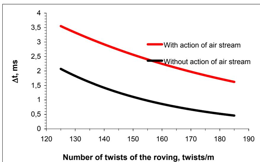
**Figure 10.** Time of destruction  $\Delta t$  as a function of the sample's twist value, in the presence of aerodynamic force acting, and without this action
