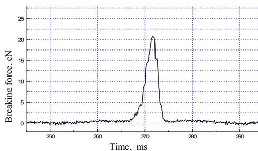
**Figure 4.** Yarn breaking diagram in dynamic conditions (slippage of fibres)
