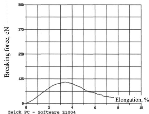
**Figure 2.** Stretching diagram of a loose textile product which loses its continuity as a result of defibration by slippage
