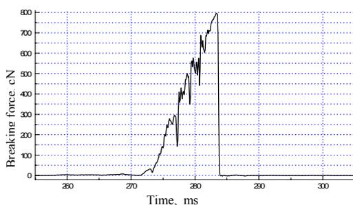
**Figure 3.** Yarn breaking diagram in dynamic conditions (breakage of fibres)
