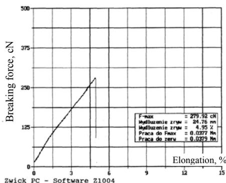
**Figure 1.** Stretching diagram of a thread which loses its continuity as a result of breakage
