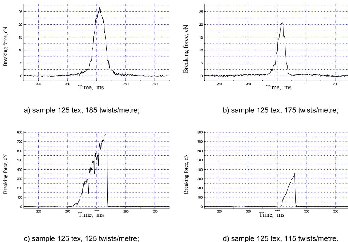
**Figure 6.** Changes of the stretching force  $F$  with time, under dynamic conditions, without air stream action, in dependence on twist value. The velocity of force applying was 5.5 m/sec
