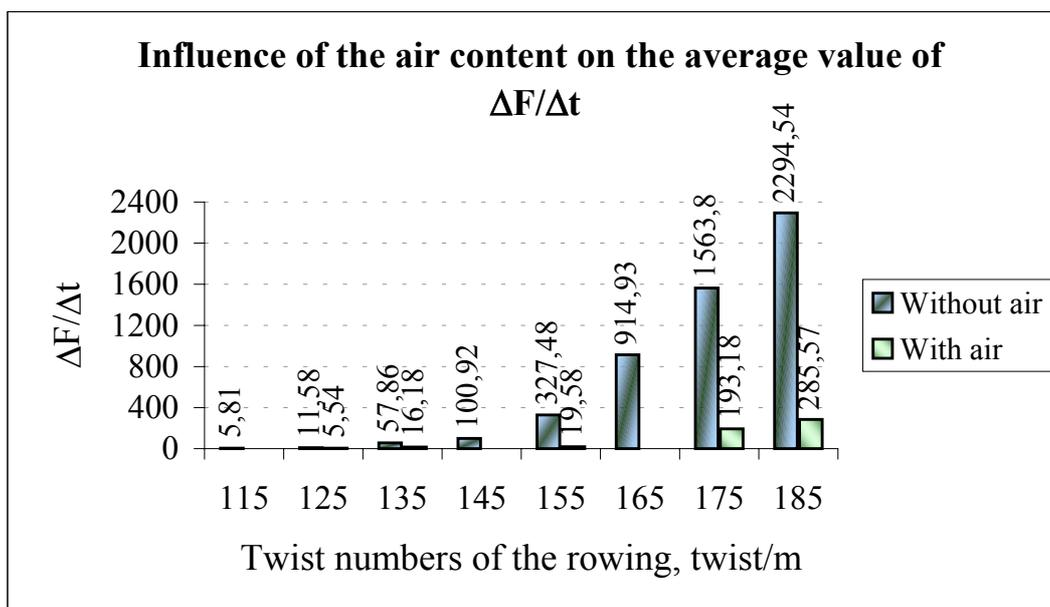
**Figure 8.** The dependence of the quotient  $\Delta F/\Delta t$  on the twist of a sample with linear density of 125 tex, subjected to the action of an air stream with velocity of 63 m/s, and of one not subjected to such an action
