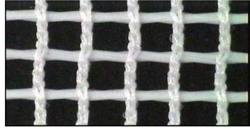
**Figure 2.** Structure of a knitted fabric destined to strengthen the pile of fibre over the needling process
