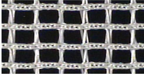
**Figure 1.** Photo of a knitted net structure before silicon carbide deposition (a selected example)
