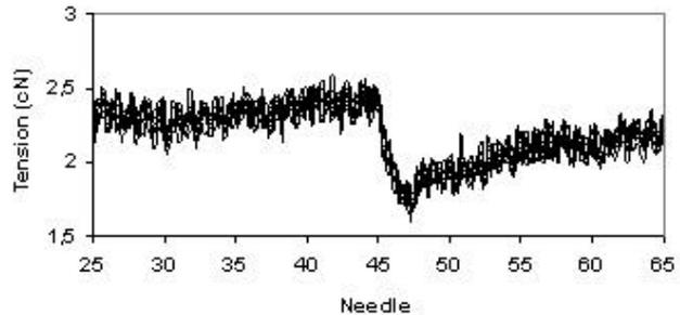
5. details for 10 revolutions: resultant waveform of a needle without its hook.
