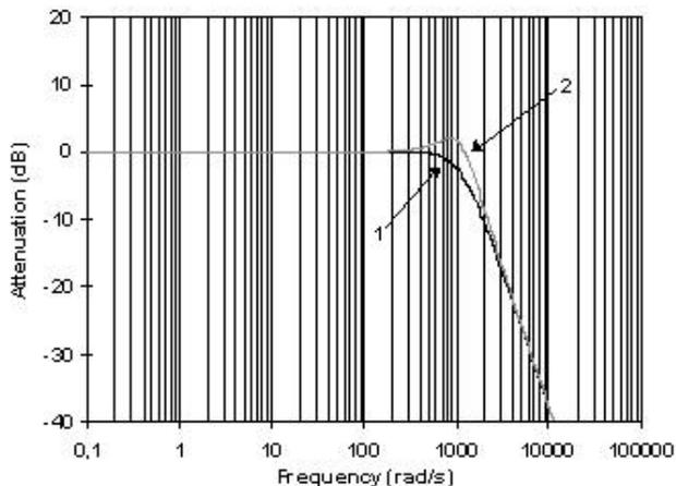
**Figure 1. Frequency response of Rothschild tension meter**
