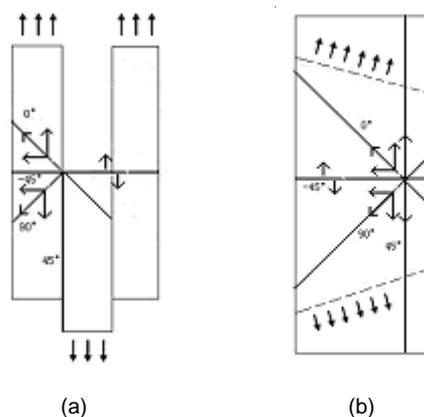
**Figure 6.** Tearing propagation resistance of the yarns in different directions (testing along +45°)
