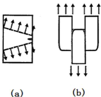
Figure 2. Different tearing methods (a)Trapezoidal, (b) Tongue Tearing
