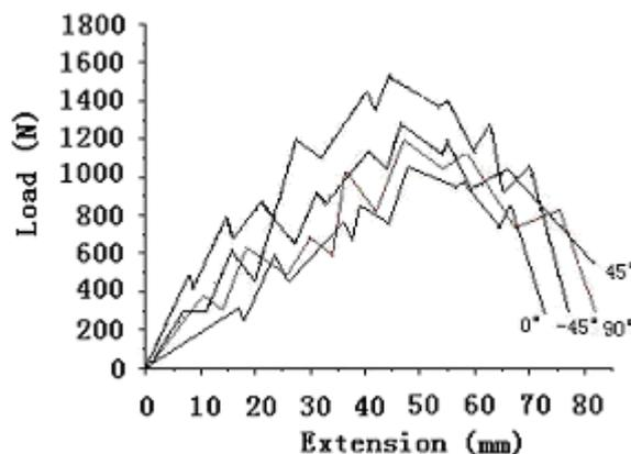
Figure 4. Typical load-extension curves under trapezoidal tearing testing condition
