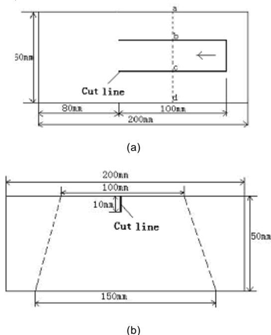
Figure 3. Dimensions of the samples (a) Trapezoidal, (b) Tongue Tearing
