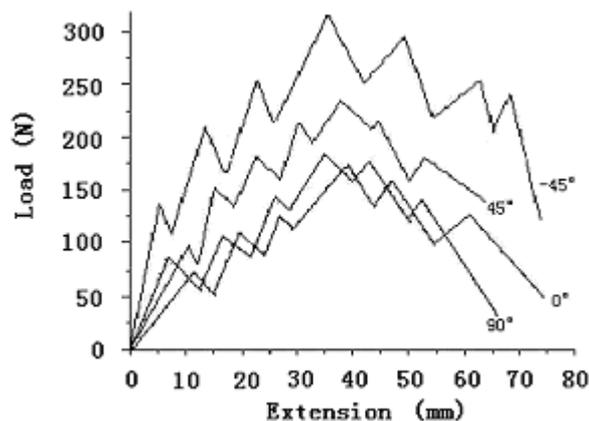
Figure 5. Typical load-extension curves under tongue tearing testing condition
