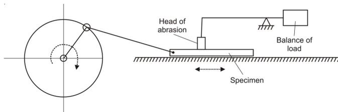
Figure 4. Mechanical principle of the "linear" abrasion tester".
