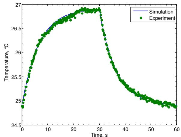
**Figure 2.** Temperature response of paper subjected to laser heating and natural cooling.
