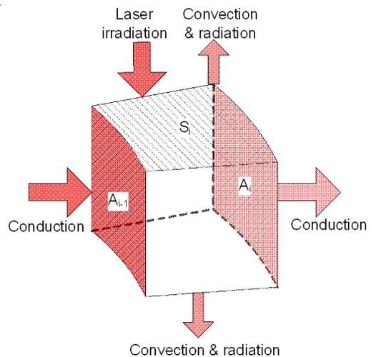
Figure 1. A control volume in paper plane for heat transfer analysis.
