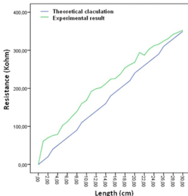
Figure 2. Resistance against length, theoretical prediction and experimental data.
