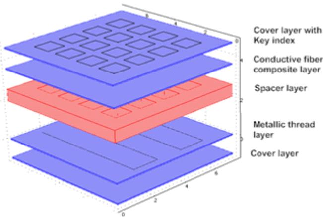
Figure 3. The construction of textile keyboard with 16 keys.
