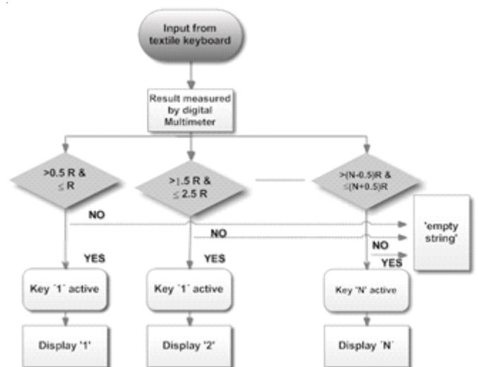
Figure 6. Flow chart of confirmation key press and display function.
