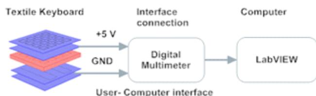
Figure 7. Overview of the keyboard testing system. There are only two interconnections between the textile keyboard and the test setup, the VCC power in and ground.
