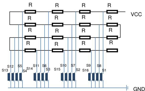
Figure 1. Keyboard equivalent circuit.
