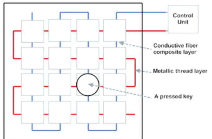
Figure 5. Top view of sensor when one key is active.
