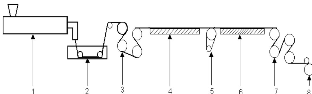
**Figure 1.** Schematic diagram of extruder and two stage drawing.
