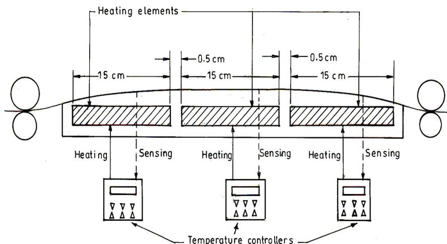
**Figure 2.** A three-element gradient heater
