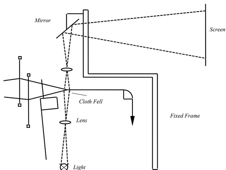
**Figure 1.** Optical method for measuring cloth fell movement
