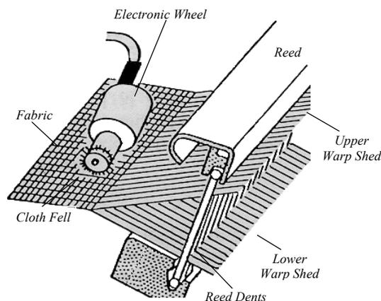
**Figure 2.** Electronic needle wheel method for measuring cloth fell movement
