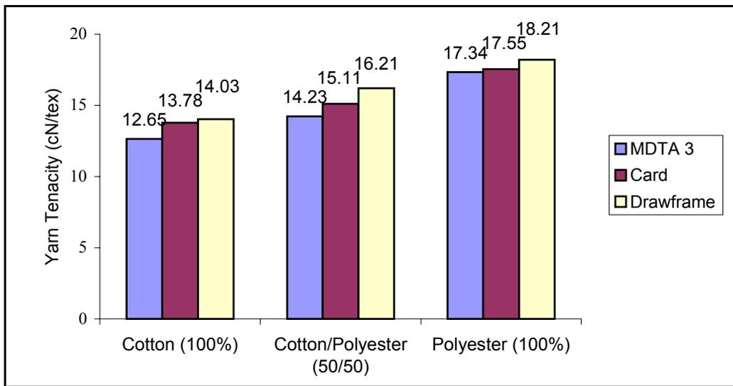
**Figure 4.** Comparison of yarn tenacity produced from MDTA 3, card, and drawframe slivers
