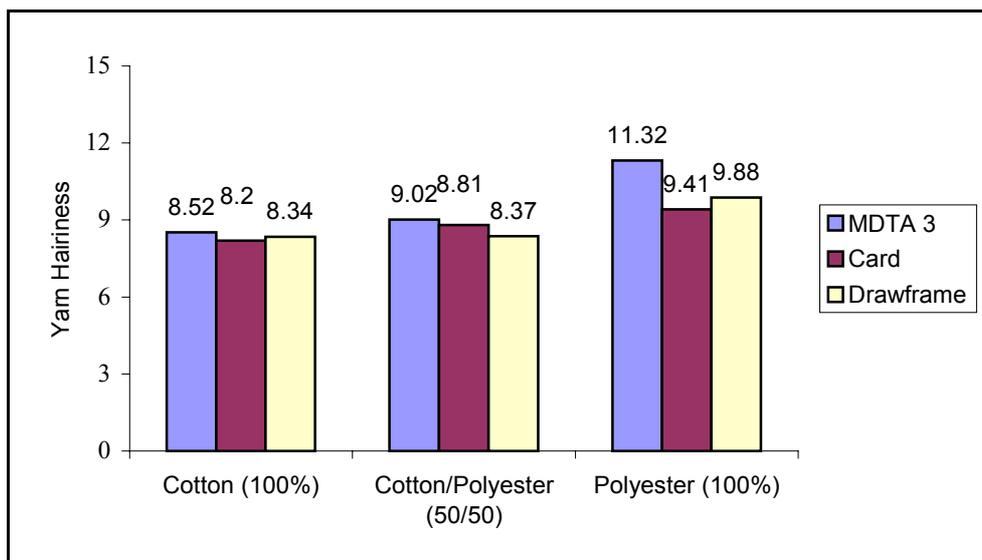
Figure 6. Comparison of yarn hairiness produced from MDTA 3, card, and drawframe slivers
