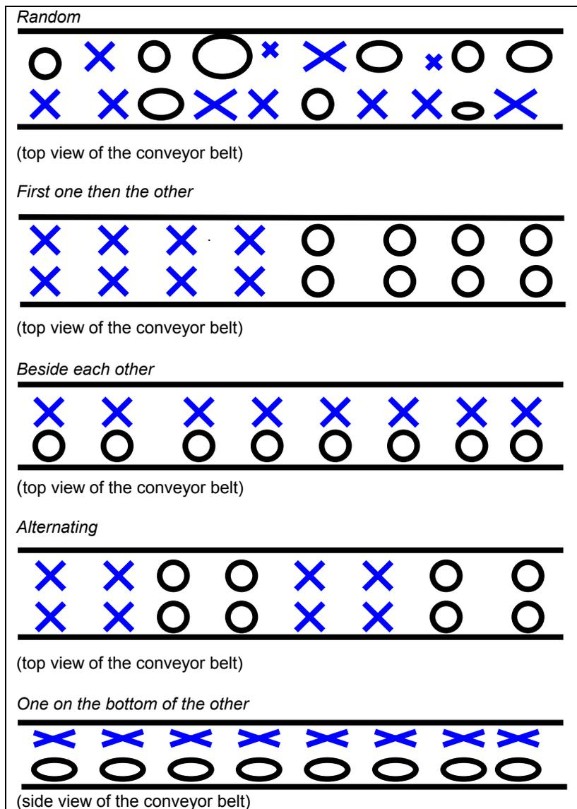
**Figure 1.** Different methods of fibre arrangement on the conveyor belt of the Uster MDTA 3 (x and o indicate two different types of fibres)
