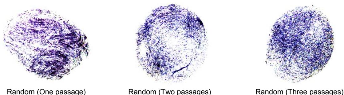
**Figure 3.** Cross-sectional view of MDTA 3 slivers produced by the *random* method of fibre blending depending on the number of passages
