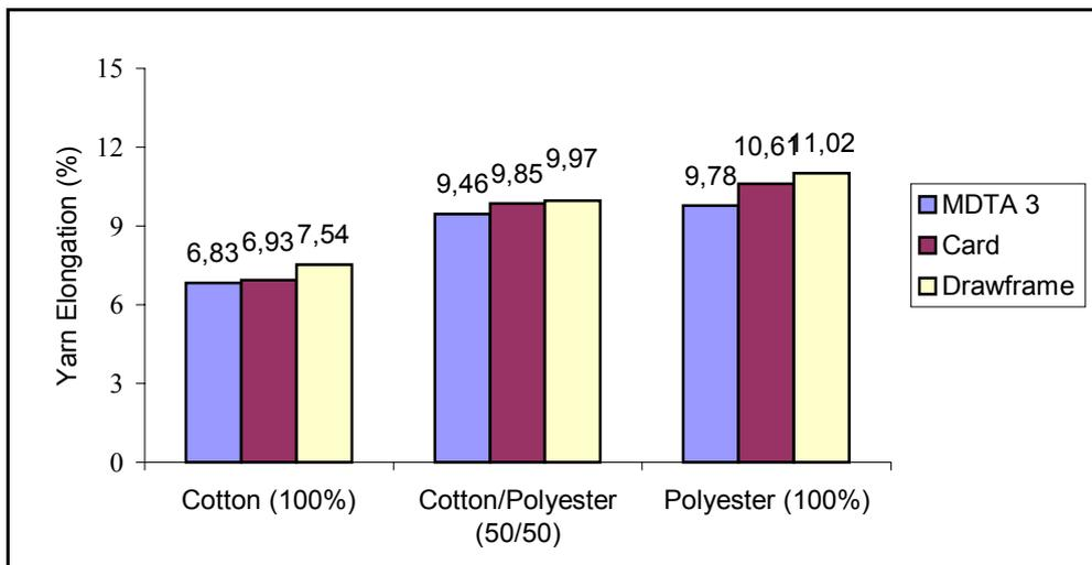
**Figure 5.** Comparison of yarn elongation produced from MDTA 3, card, and drawframe slivers
