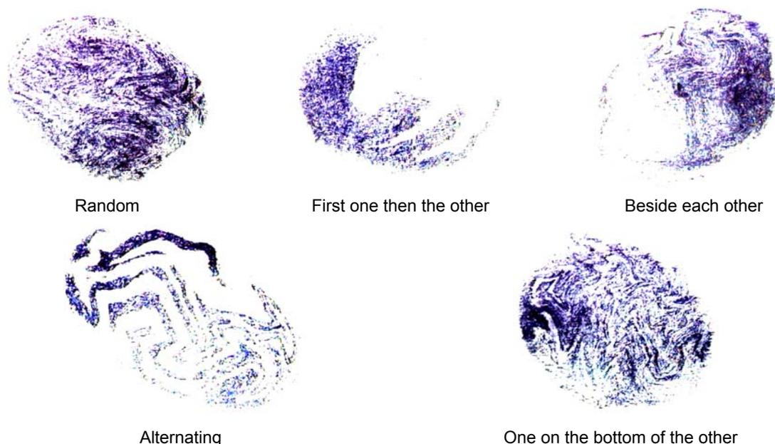
**Figure 2.** Cross-sectional view of MDTA 3 slivers produced by different blending methods
