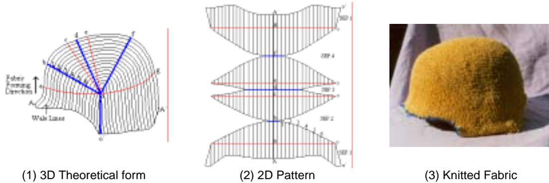
**Fig. 1.** Helmet form produced with aramid fibres
