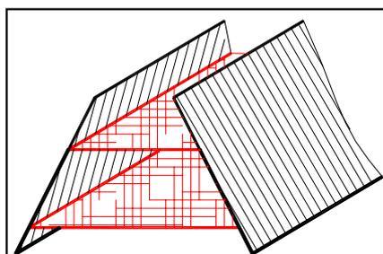
Fig. 6. Sandwich fabric with layers of different length
