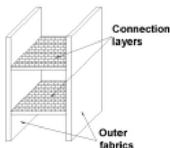
Fig. 4. Sandwich structure
