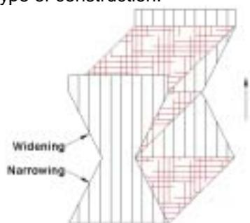
Fig. 9. Sandwich fabric with shaped outer fabrics
