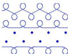
**Figure 2.** Double woven rib knitted with DREF yarns
