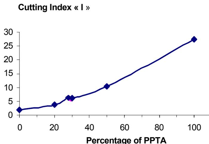
**Figure 3.** Cutting performances of DREF yarns
