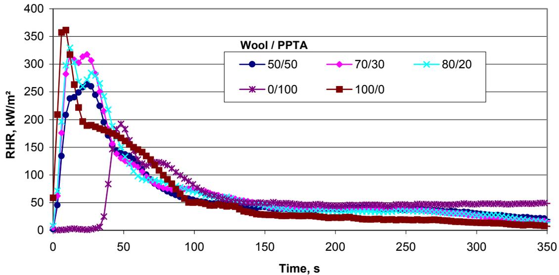
**Figure 4.** RHR curves of blends wool/PPTA (external heat flux = 75 kW/m<sup>2</sup>)
