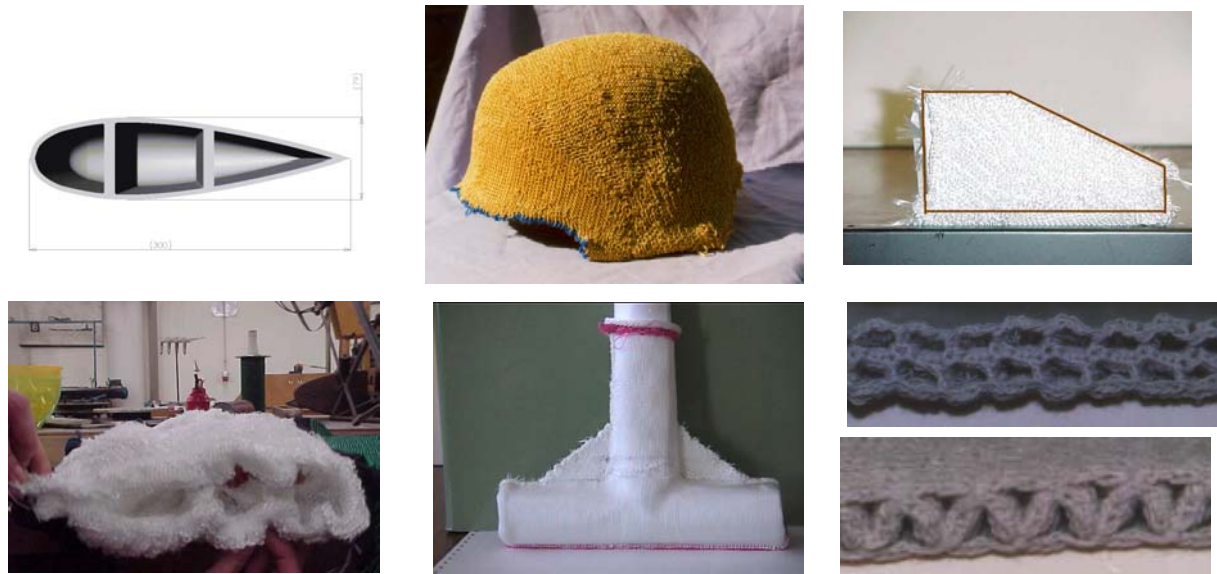
Figure 1. Examples of the versatility of weft knitting technology for the production of 3D complex shaped fabrics for composite reinforcement
