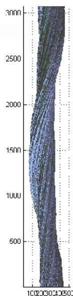
**Figure 5.** Image of surface topology of an acrylic yarn processed with the virtual surface profiler
