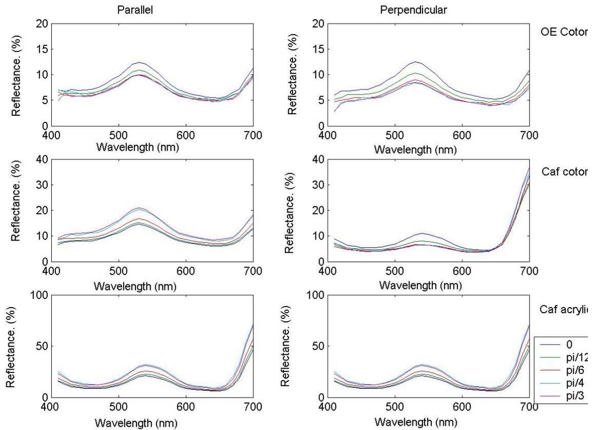
**Figure 6.** Examples of reflectance spectra for the three sample sets and the two instrumental configurations
