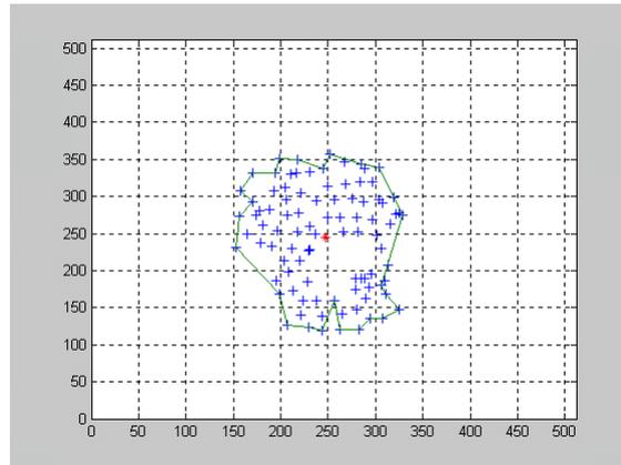
**Figure 3.** Yarn contour (straight line) and fibre centre positions (+) from an acrylic yarn
