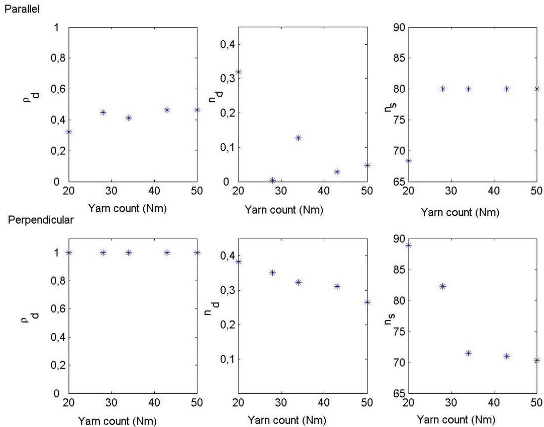
**Figure 7.** Evolution of Lafortune model's parameters as a function of the yarn count for the sample set CAF cotton
