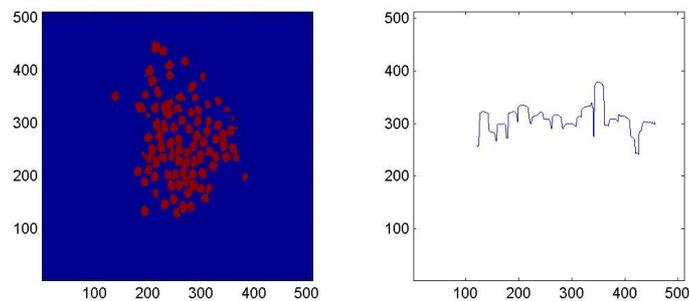
**Figure 4.** Yarn profile obtained from the yarn transversal section image
