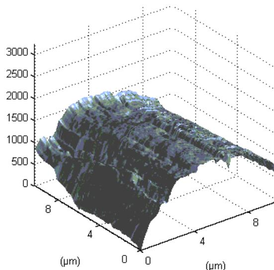
**Figure 1.** AFM image of surface topology of an acrylic fibre
