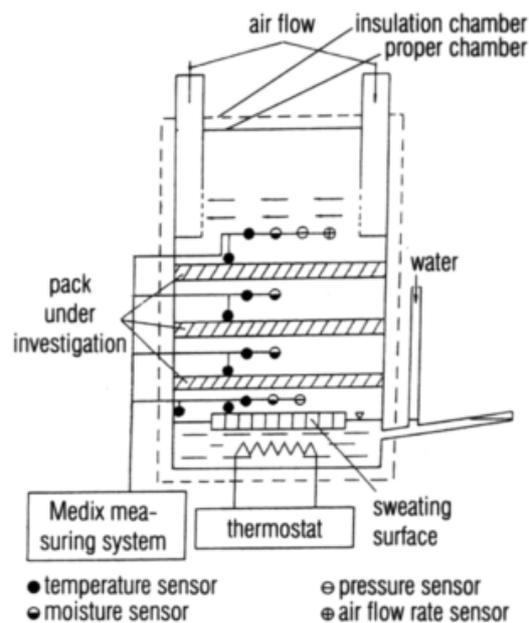
**Figure 2.** A schema of the apparatus for the assessment of moisture transport through flat textiles
