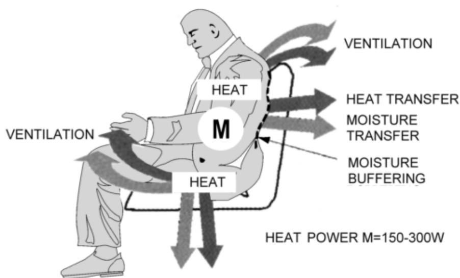
**Figure 1.** Heat and moisture streams in an upholstery car seat
