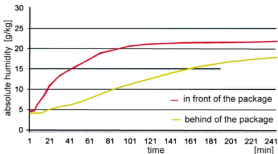
**Figure 4.** Absolute humidity changes as a function of time for the outside layers of package 'c'
