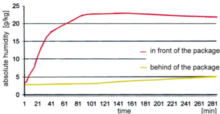
Figure 3. Absolute humidity changes as a function of time for package 'c'
