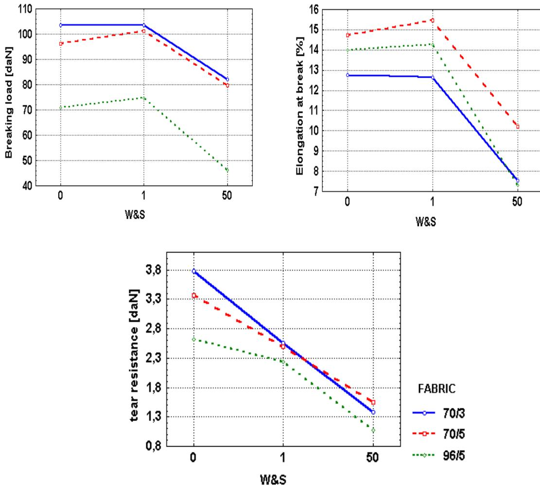
**Figure 2:** Mechanical parameters of fabrics before and after process of washing and sterilisation
