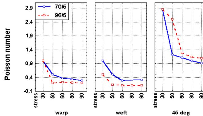
Figure 7: Poisson number at different stress levels
