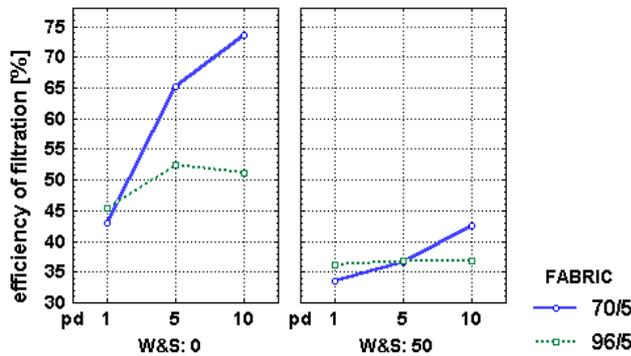
Figure 4: Efficiency of filtration of sodium chloride and silicon dioxide aerosols
