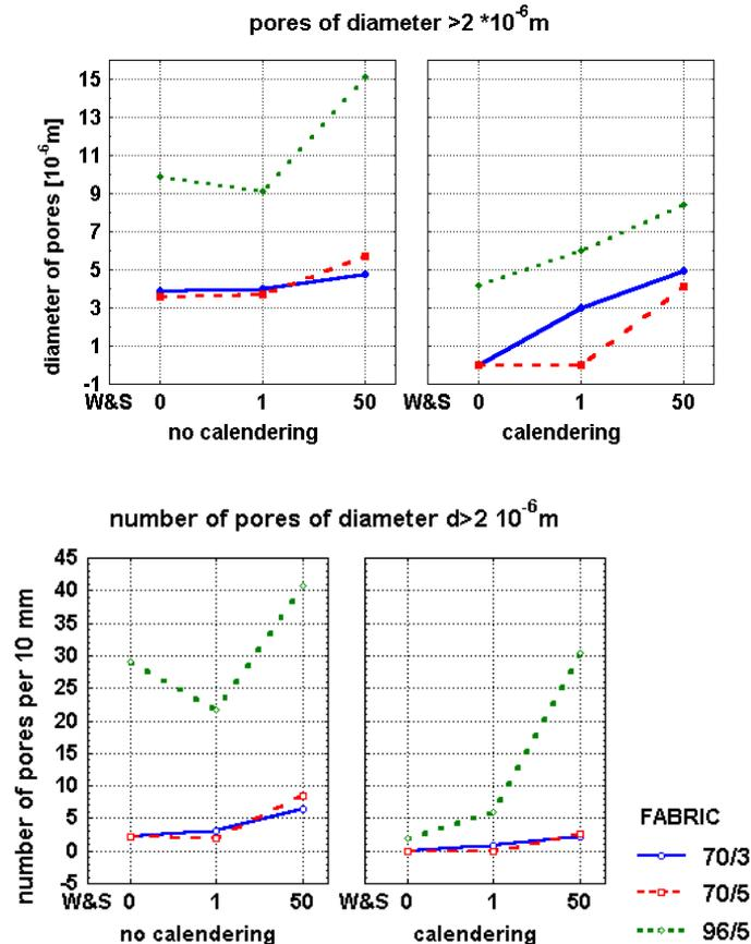
Figure 5: Fabric porosity by image analysis
