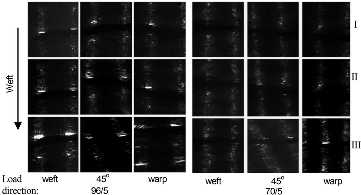
**Figure 6:** The effect of pulsatory loading on the fabric porosity. Images of the same 0.5 mm-long sections of 96/5 and 70/5 fabrics: I – before loading, II – after 50 cycles of 30 daN load, III – after the breakage.
