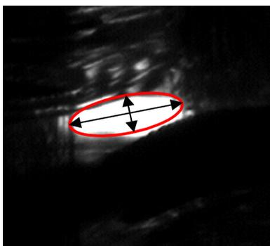
**Figure 1:** Measurement of the pore size
