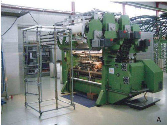
Figure 3. Double-needlebar raschel machine (A); developed yarn supplying system (B).
