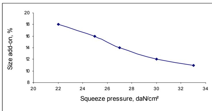
**Figure 2.** influence of squeeze pressure on size add-on.
