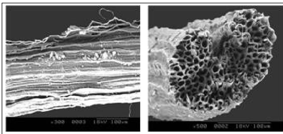
**Figure 3.** Longitudinal and cross-section views of an agave *Americana L.* fibre
