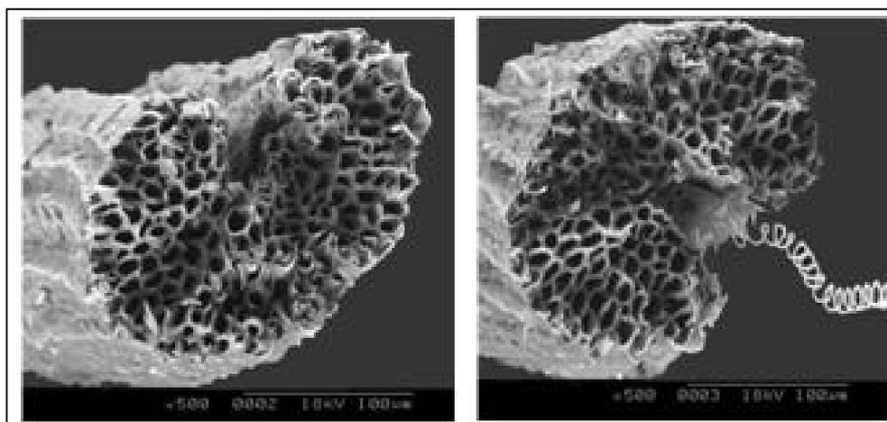
Figure 5. The tensile fracture morphology of an agave *Americana L.* fibre
