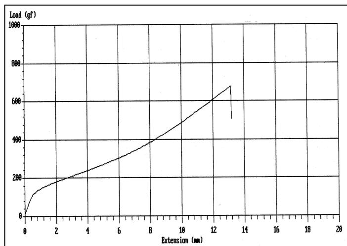
Figure 4. Stress-strain curve of an agave *Americana L.* fibre
