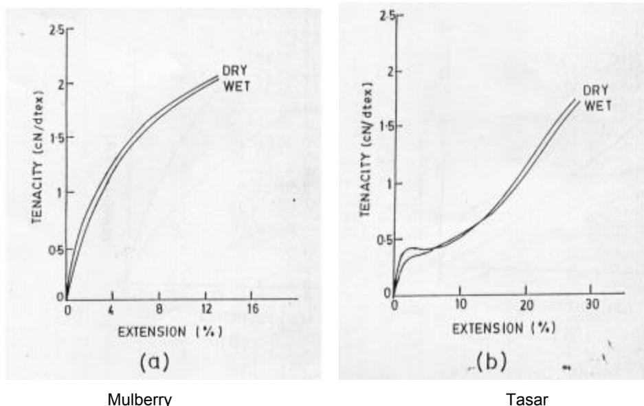
Figure 1. Stress-strain behaviour of fully degummed silk filaments (Fibroin) in dry and wet conditions
