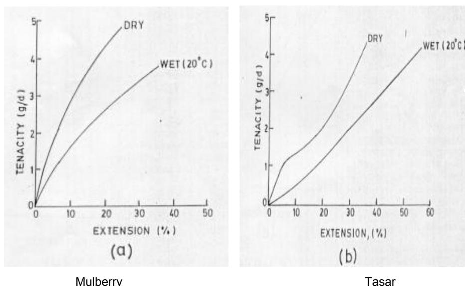
Figure 2. Stress-strain behaviour of silk yarns in dry and wet conditions (adapted [1])
